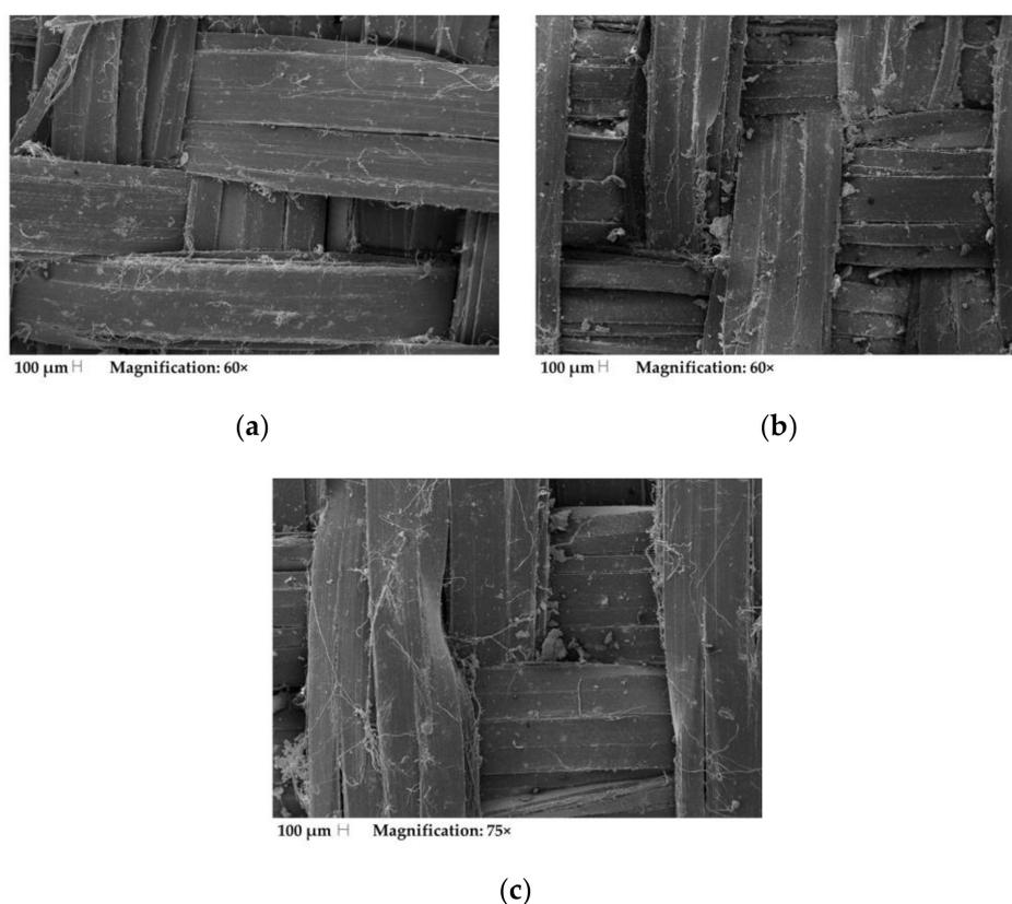
**Figure 14.** W1 SEM (magnification:  $60\times$  and  $75\times$ ). (a) Virgin sample. (b) Sample with less permittivity reduction (scenario 0C). (c) Sample with high permittivity reduction (scenario -1B).
