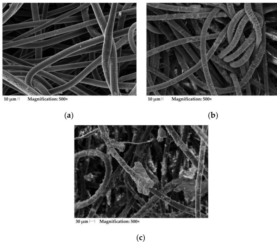
**Figure 13.** NW2 SEM (magnification: 500×). (a) Virgin sample. (b) Sample with less permittivity reduction (scenario 1C). (c) Sample with high permittivity reduction (scenario -1C).
