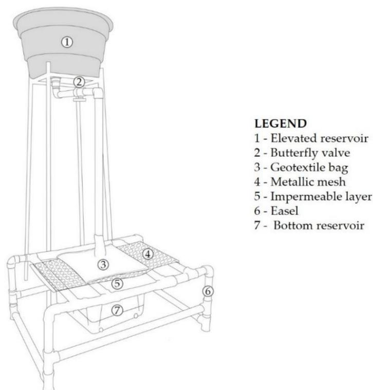
**Figure 3.** Geotextile tube dewatering test scheme.
