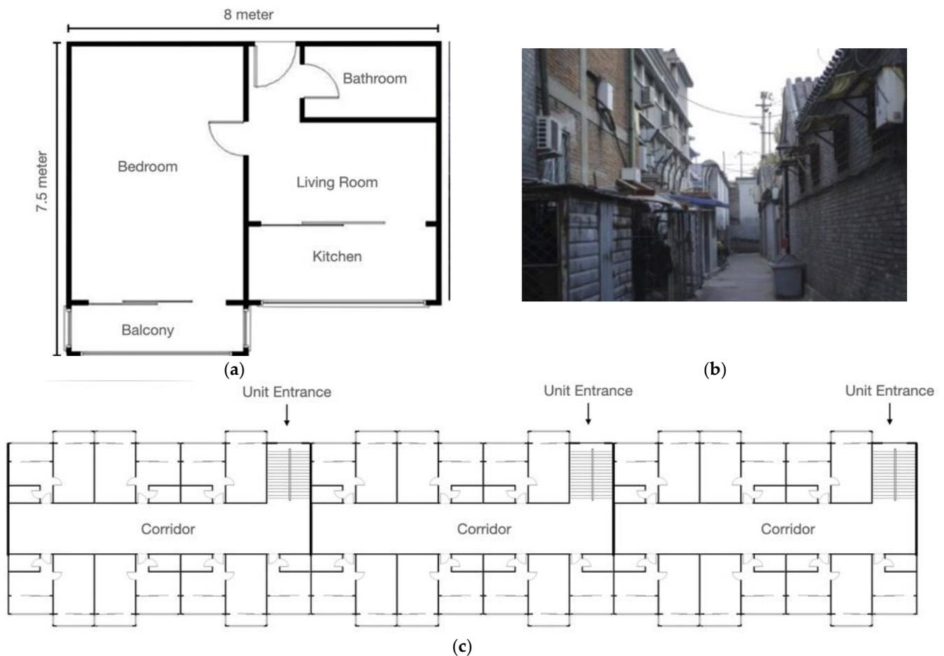
Figure 10. Modern apartment and its layout. Top left image shows the apartment layout (a); top right image presents the building design (b); and down image illustrates the floor plan of the building (c).
