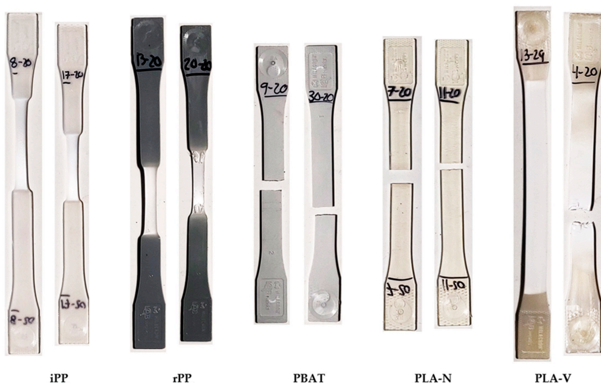
Figure 5. Images of representative tested specimens for the (left) highest and (right) lowest specimens for each of the five investigated materials as indicated in the structural performance plot of Figure 4.
