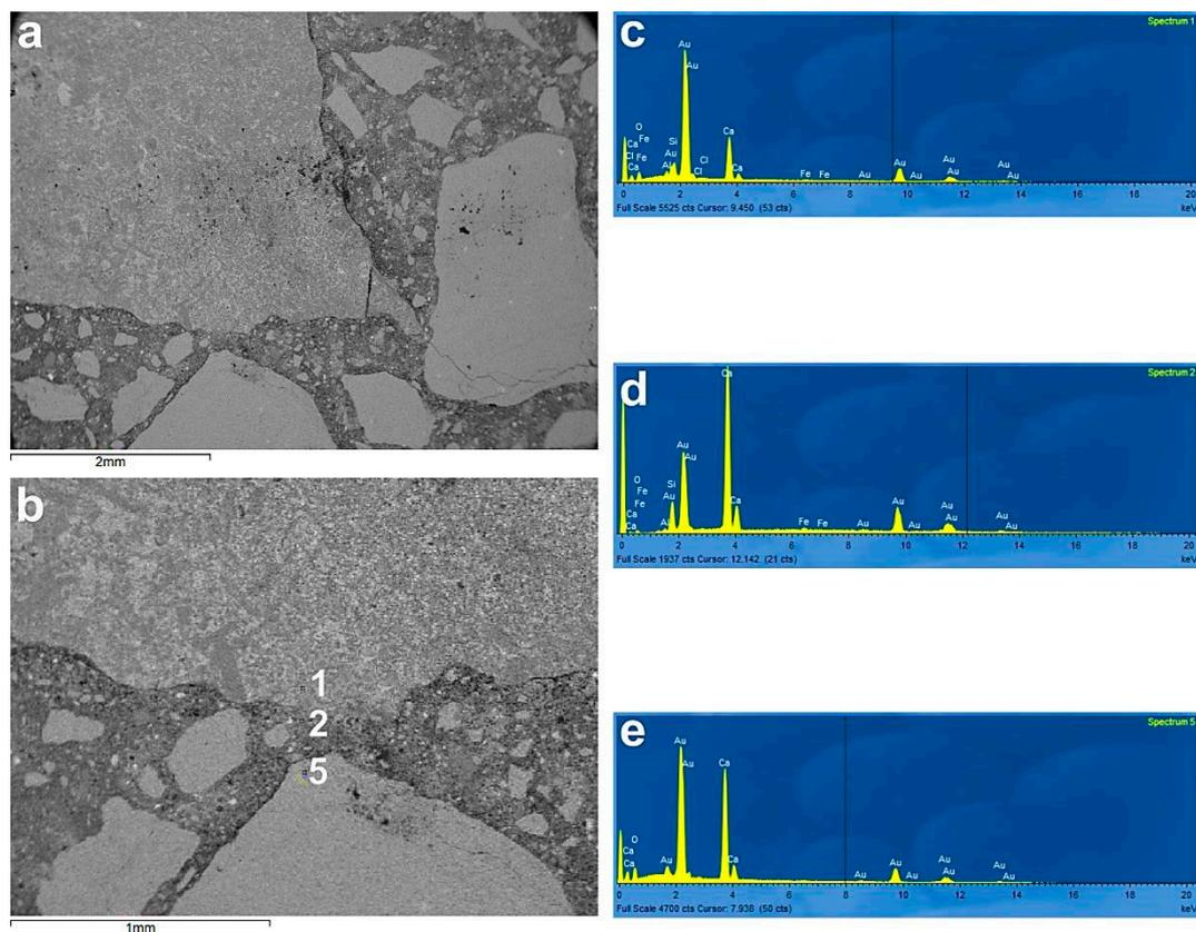
**Figure 11.** (a,b) Back scattered image of a concrete specimen; (c–e) SEM-EDX spectra from the interface of an aggregate particle with the cement paste from the spots 1, 2, 5 as shown in Figure 11b.
