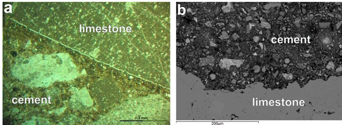
**Figure 6.** (a) Photomicrograph (sample SOA) and (b) secondary electron image (sample SOB) showing reference tested concretes with good cohesion between limestone aggregate grains and cement paste.
