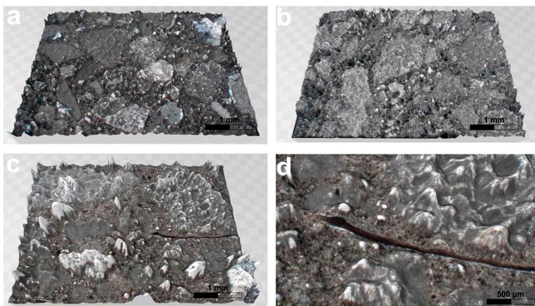
**Figure 10.** (a–d): 3D depiction of the investigated concrete specimens.
