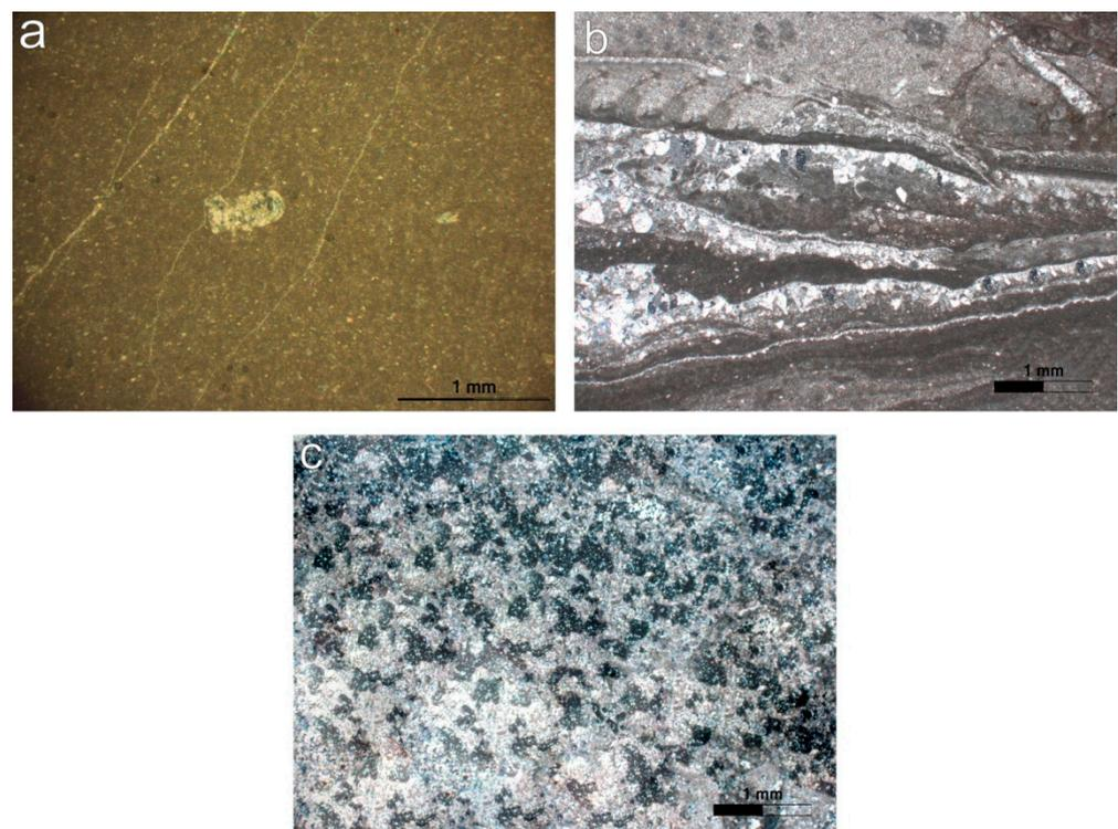
**Figure 2.** Photomicrographs of natural aggregates and animal bones used as aggregates in crossed nicols showing: (a) micritic limestone; (b) zoned bone (goat) with calcite; (c) amorphous bone (sheep) with cryptocrystalline calcite.
