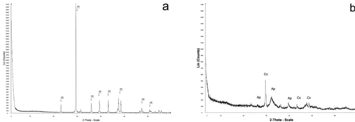
Figure 3. X-ray diffraction pattern of: (a) limestone; (b) goat's bone (Cc: calcite, Ap: apatite).
