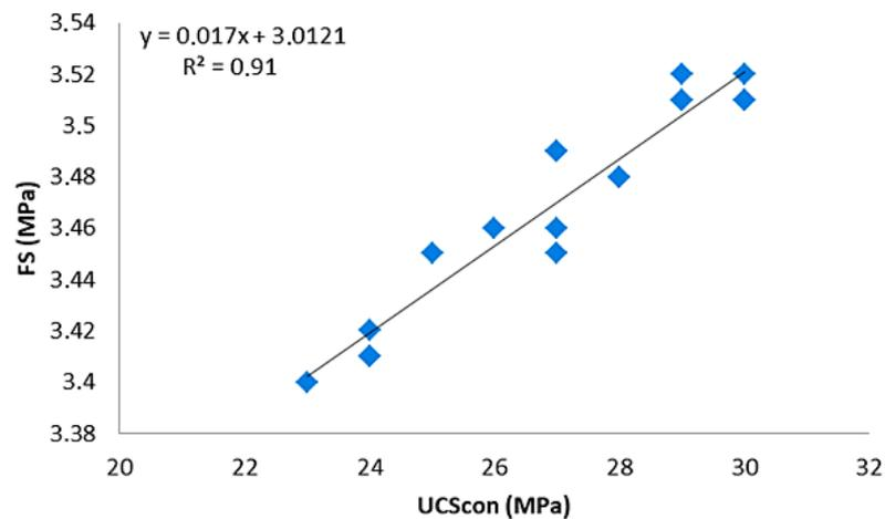
**Figure 5.** Uniaxial compressive strength (UCScon (MPa)) vs. the flexural strength (Fs (MPa)) of the produced concrete specimens.
