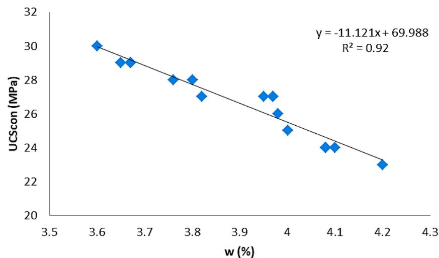
**Figure 8.** Moisture content ( $w$  (%)) of animal bones vs. the uniaxial compressive strength (UCScon (MPa)) of the produced concrete specimens.
