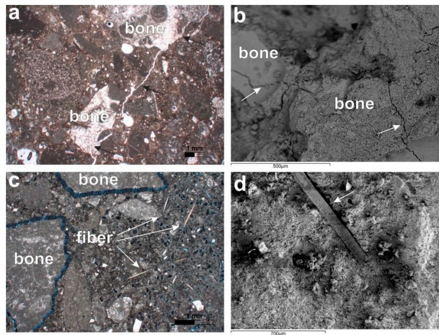
**Figure 7.** Photomicrographs of representative tested concretes showing: (a) animal bone aggregates (parallel nicols, sample S1A); (b) animal bone aggregates (sample S1B); (c) animal bone aggregates coating with quartz primer and human hair fibers (crossed nicols, sample S2A). Back scattered electron images showing microstructures at the interface between cement paste; (d) human hair fiber (sample S2B).
