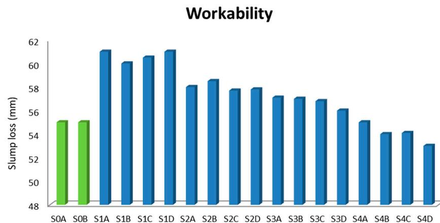
Figure 4. Chart of the workability of the concrete specimens (with the green color representing the reference concrete specimens).
