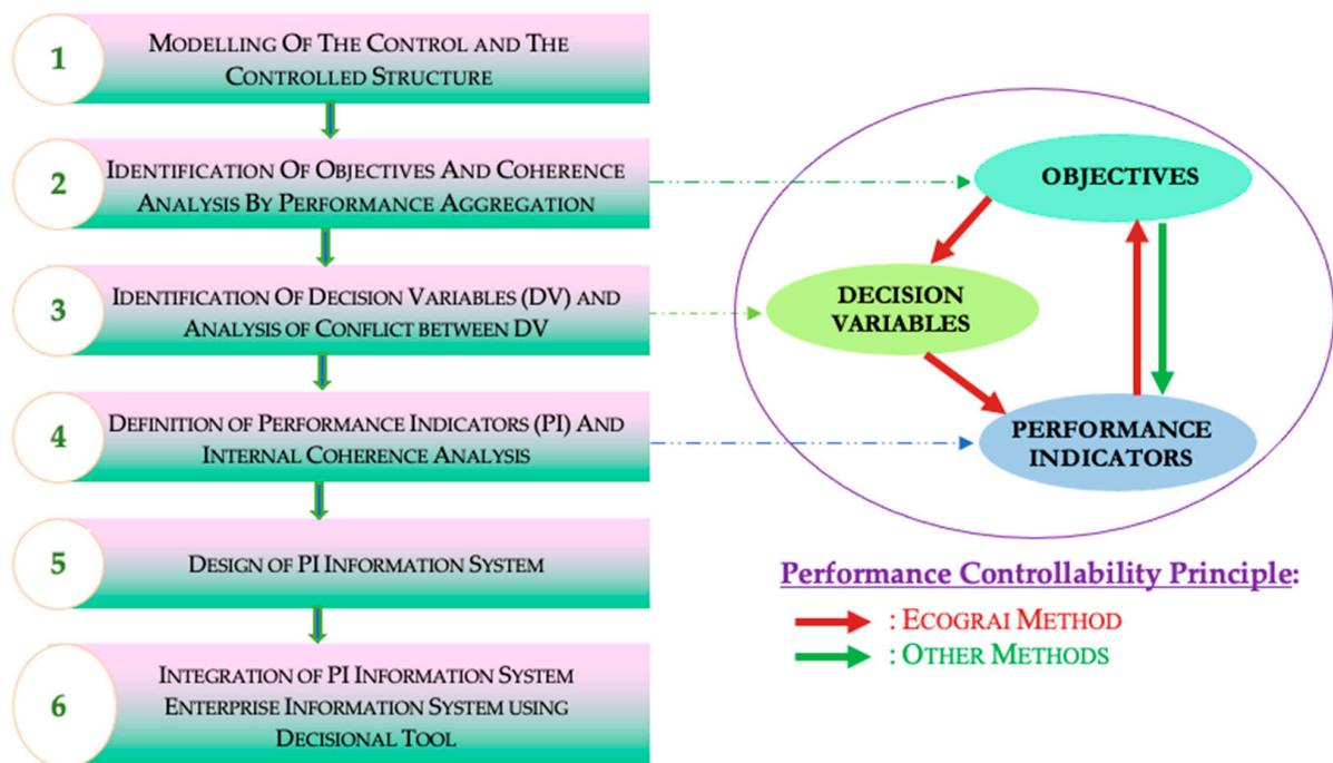
**Figure 2.** Six steps of the ECOGRAI method of indicators design and its performance controllability principle (originality). Source: Elaborated from [7,40].
