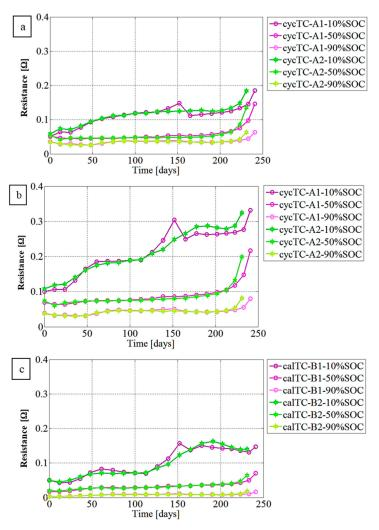
**Figure 6.** Internal Li–SBs resistance of discharge cycling aging for (**a**) 1 s, (**b**) 30 s (**c**) (30-1) s for 10%, 50%, at 90% SOCs and C-rate of 0.5.
