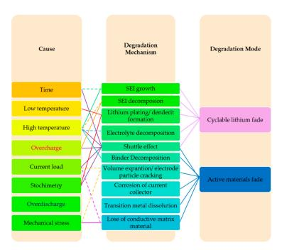
**Figure 2.** Network diagram of the causes and mechanisms of lithium-sulfur battery degradation. (Solid lines: indicates the proven items in the literature. Dashed lines: are based on the results of the analysis of lithium-ion batteries and are yet to be proven) [9,23–30].
