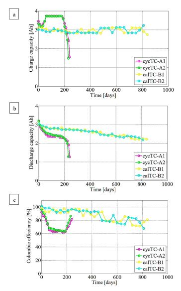
**Figure 3.** Cycling performance profiles include (**a**) charge capacity, (**b**) discharge capacity, (**c**) coulombic efficiency.
