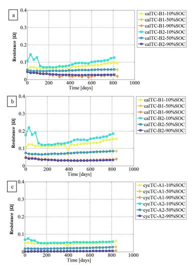
**Figure 7.** Internal Li–SBs resistance of discharge calendar aging (a) 1 s, (b) 30 s (c) (30-1) s for 10%, 50%, at 90% SOCs and C-rate of 0.5.
