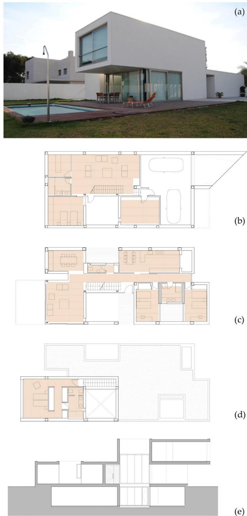
**Figure 2.** Description and distribution of the detached house. (a) View of the house on its northeast facade. Outdoor porch of the living room and pool; (b) basement; (c) ground floor; (d) first floor; (e) longitudinal section through the courtyard. The basement acts as a passive bioclimatic system.
