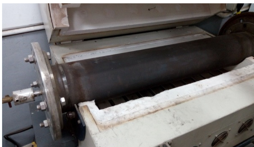
Figure 7. Photograph of prototype cyclone-type rotary kiln.
