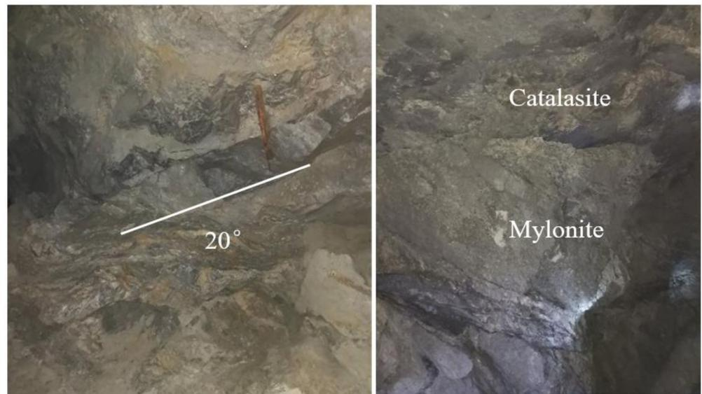
Figure 3. Picture of occurrence of ore body in Miao-ling gold mine.
