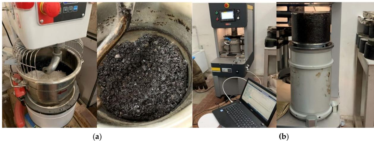
**Figure 4.** (a) Asphalt mixing phase and (b) gyratory compaction.
