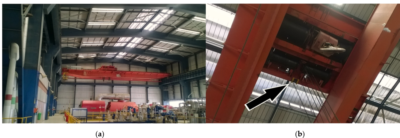
Figure 3. Case-study: (a) Overhead crane and working area; (b) Location of the anti-collision device.
