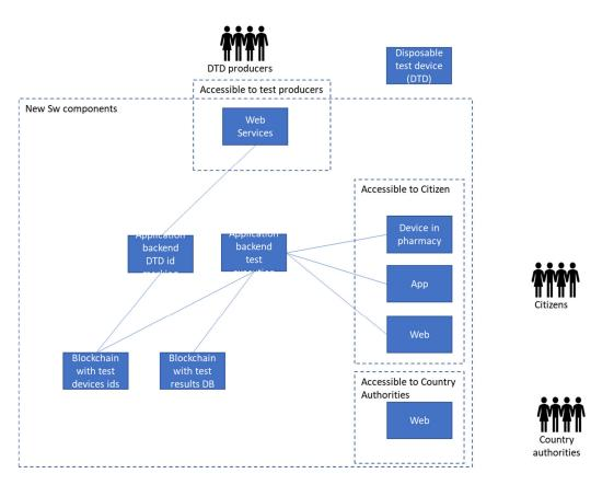
Figure 1. Vpassport high-level architecture.
