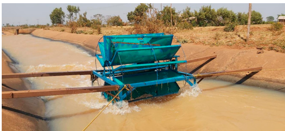
Figure 1. Water turbine (approximately 1.4 kW of power output) on the Koga canal located in the region surrounding the study domain.
