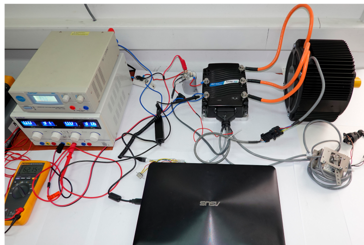
Figure 6. Curtis 1236SE three phase inverter connected to electric motor for preliminary test.
