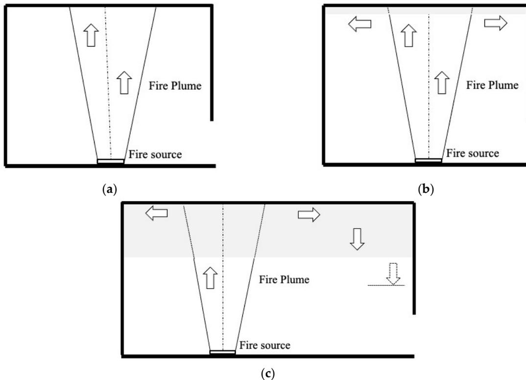
**Figure 1.** Schematic depiction of smoke filling an enclosure [29,36,40], where (a) is development of fire plume in enclosure, (b) is ceiling jet, and (c) is smoke layer descent in enclosure without smoke vents.
