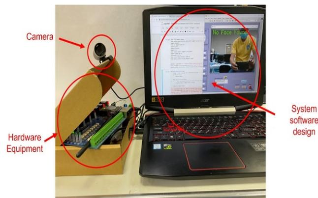
**Figure 16.** The appearance of the designed system in practice.
