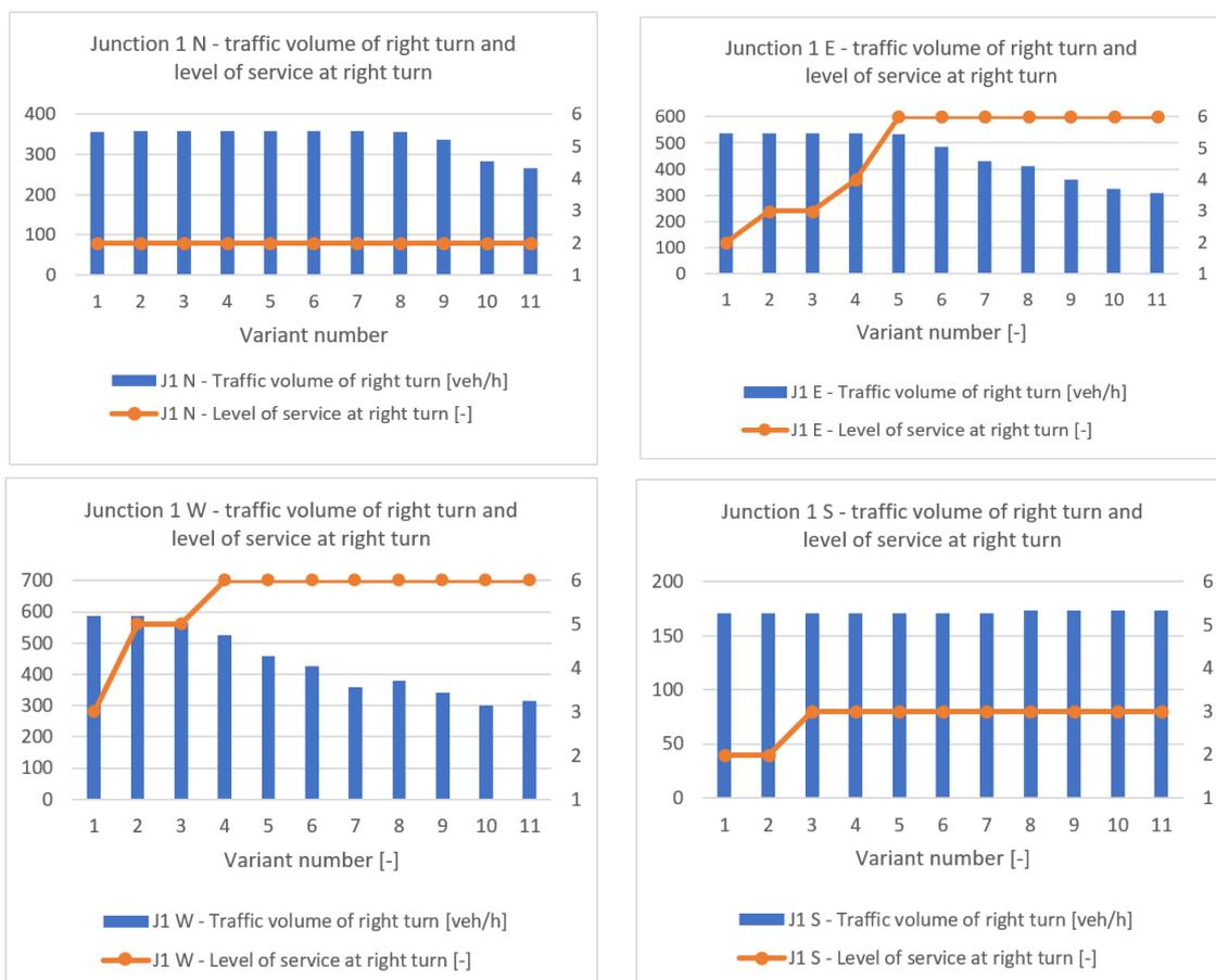
Figure 5. LOS analysis of Junction 1 right turns—comparison.
