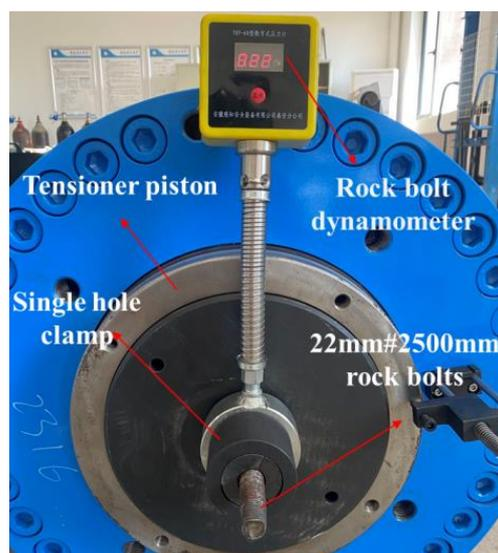
**Figure 14.** Bolt dynamometer testing.
