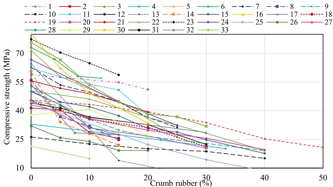
**Figure 4.** Variation of compressive strength of SCC made with different replacement levels of CR: 1 [50], 2 [30], 3 [45], 4 [43], 5 [4], 6 [47], 7 [31], 8 [48], 9 [51], 10 [52], 11 [46], 12 [68], 13 [7], 14 [66], 15 [16], 16 [18], 17 [64], 18 [38], 19 [19], 20 [71], 21 [65], 22 [62], 23 [53], 24 [60], 25 [44], 26 [49], 27 [57], 28 [58], 29 [67], 30 [56], 31 [61], 32 [72], 33 [54].
