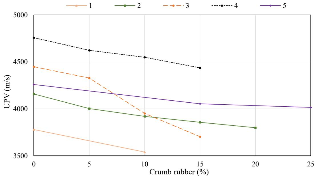
Figure 15. Variation of UPV of SCC made with different replacement levels of CR: 1 [4], 2 [49], 3 [48], 4 [53], 5 [60].
