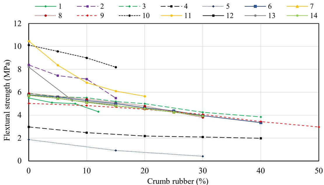
**Figure 10.** Variation of flexural strength of SCC made with different replacement levels of CRs: 1 [47], 2 [48], 3 [51], 4 [52], 5 [7], 6 [16], 7 [18], 8 [38], 9 [19], 10 [53], 11 [56], 12 [61], 13 [72], 14 [54].
