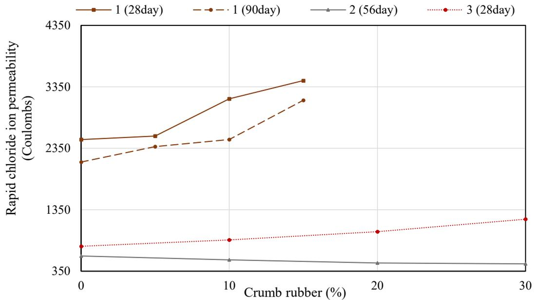
**Figure 19.** Variation of rapid chloride permeability in coulombs of SCC with different replacement levels of CR: 1 [15], 2 [64], 3 [38].
