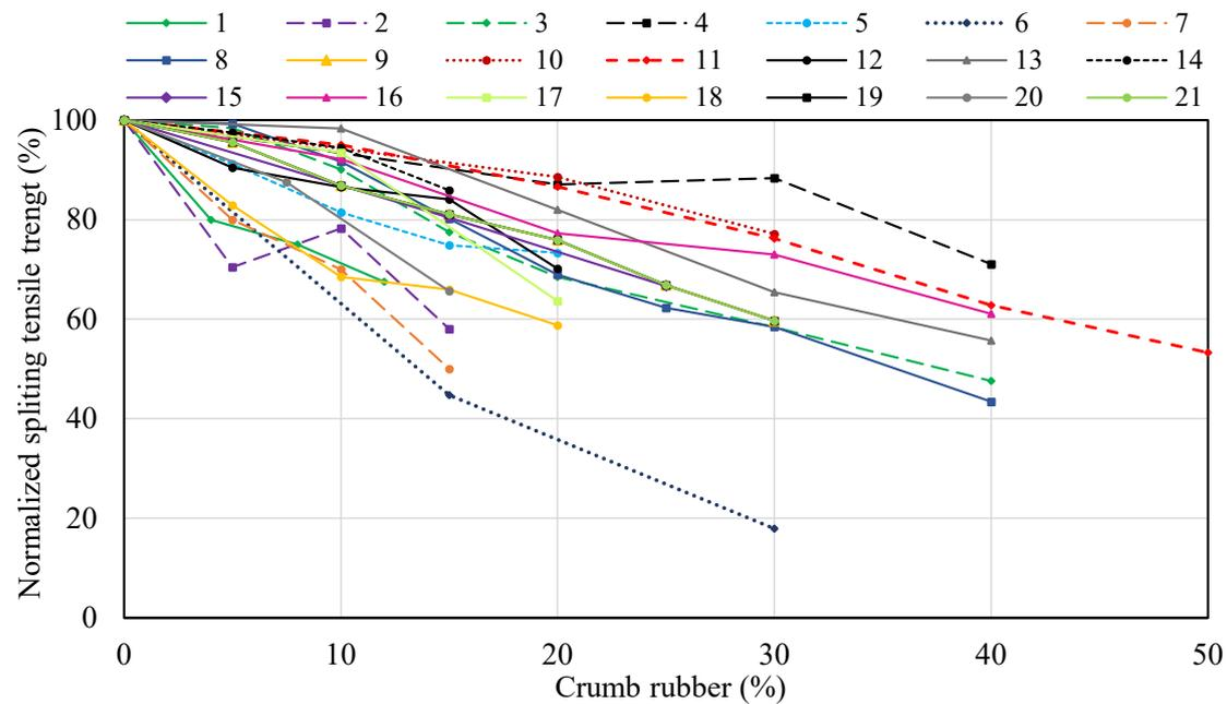
**Figure 7.** Normalized percentage of splitting tensile strength: 1 [47], 2 [48], 3 [51], 4 [52], 5 [46], 6 [7], 7 [66], 8 [16], 9 [18], 10 [38], 11 [19], 12 [65], 13 [62], 14 [53], 15 [60], 16 [57], 17 [67], 18 [56], 19 [61], 20 [72], 21 [54].
