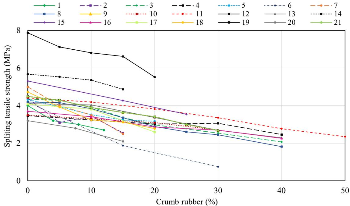
**Figure 6.** Variation of splitting tensile strength of SCC made with different replacement levels of CR: 1 [47], 2 [48], 3 [51], 4 [52], 5 [46], 6 [7], 7 [66], 8 [16], 9 [18], 10 [38], 11 [19], 12 [65], 13 [62], 14 [53], 15 [60], 16 [57], 17 [67], 18 [56], 19 [61], 20 [72], 21 [54].
