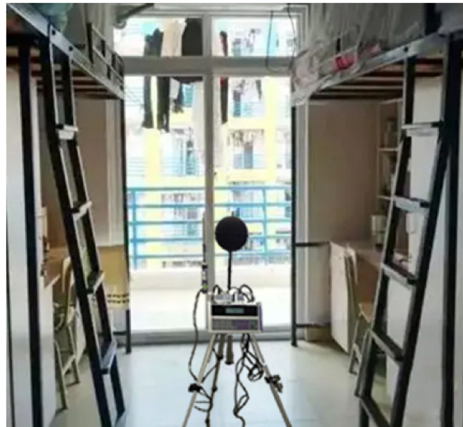
Figure 2. Field measurement for the indoor thermal environment.
