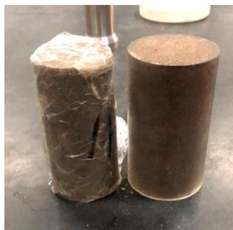
**(b)****Figure 3.** Compacted OMDS samples: (a) compaction tool; (b) OMDS samples.
