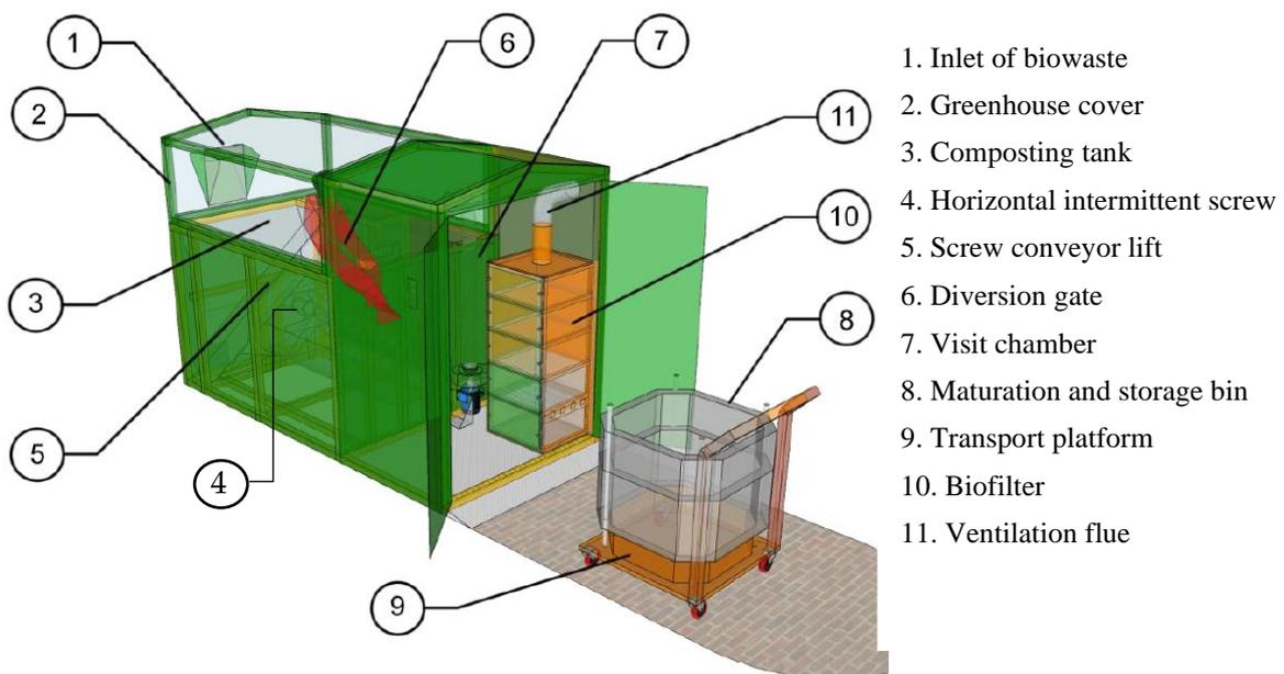
Figure 3. Solar mechanical composter (Incotech Model SMEC-3).
