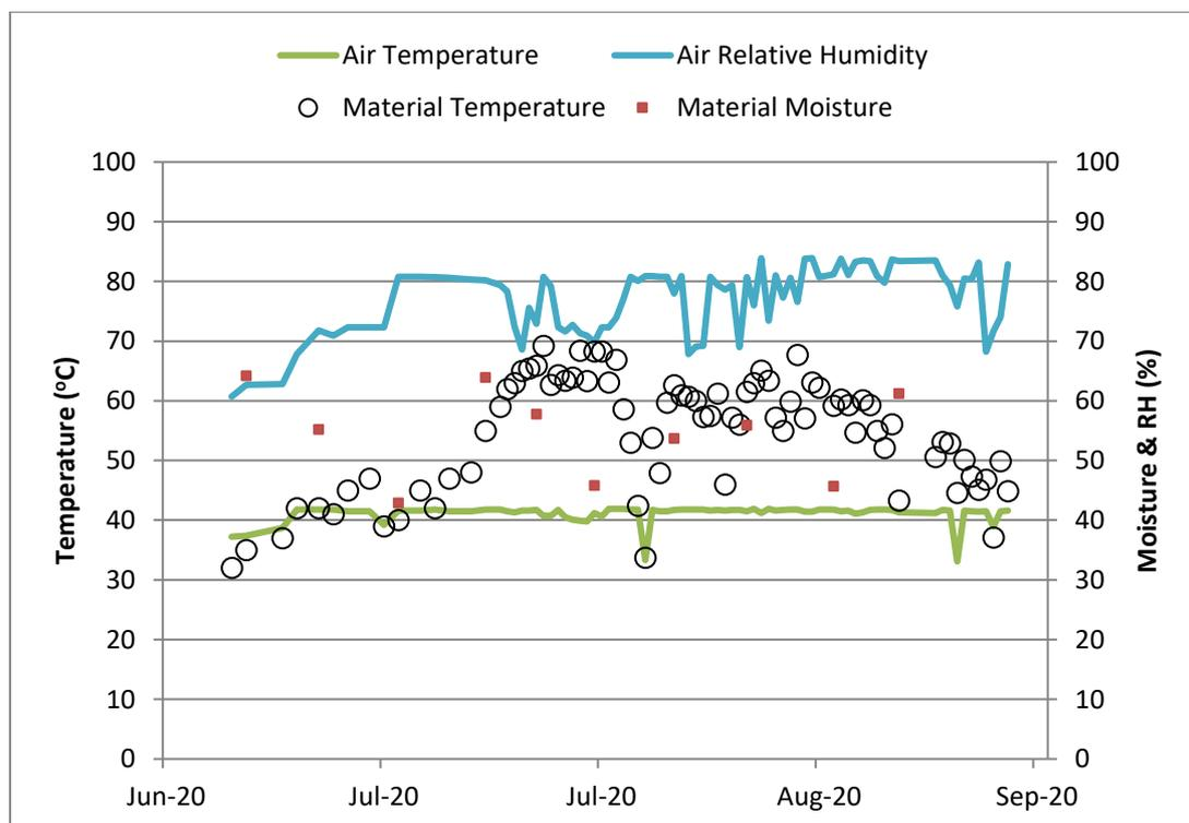
**Figure 5.** Temperature and moisture variation during composting experiment.
