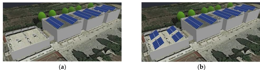
**Figure 4.** PV plant in the rooftop of the Episkopi high school building: (a) Scenario E1 and (b) Scenario E2.
