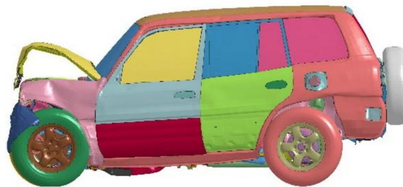
**Figure A2.** Simulation results of the frontal deformation of the SUV when impacting a rigid wall at 56 km/h speed.
