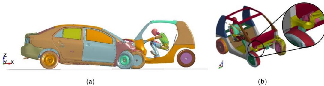
**Figure 9.** Full-frontal impact collision between the L7e vehicle and sedan: (a) vehicle deformations during the crash; (b) the deformed shape of the upper beam after the crash.
