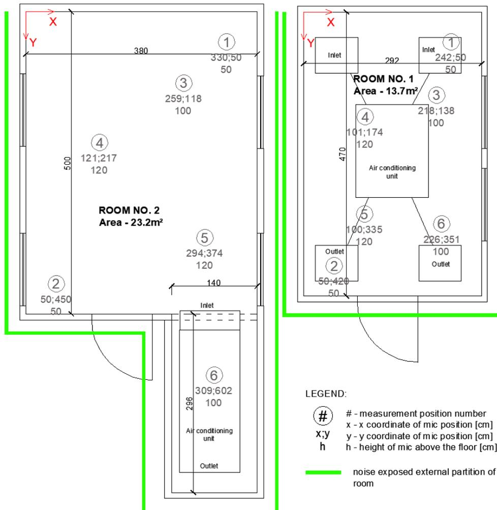
Figure 2. Plan of two mock-up rooms located inside the industrial hall.
