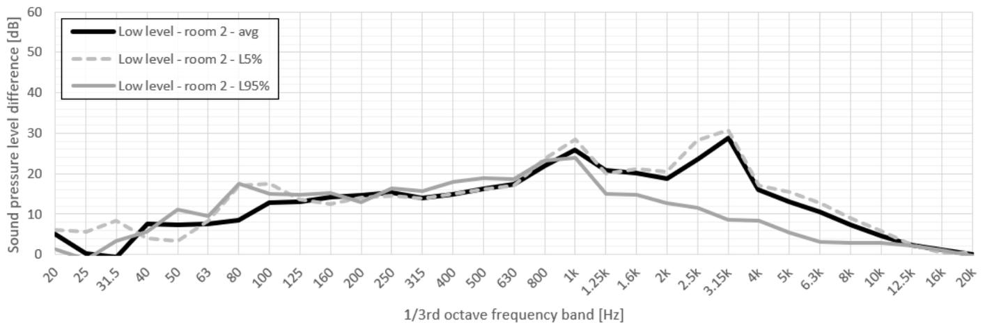
**Figure 13.** The estimated level difference between the hall and large mock-up room 2 during the low-level period with equivalent and statistical levels of L5% and L95% using Formula (2).
