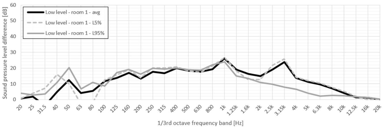
**Figure 11.** The estimated level difference between the hall and small mock-up room 1 during the low-level period with equivalent and statistical levels of L5% and L95% using Formula (2).
