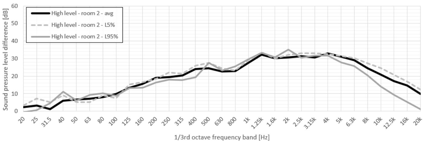
**Figure 12.** The estimated level difference between the hall and large mock-up room 2 during the high-level period with equivalent and statistical levels of L5% and L95% using Formula (2).
