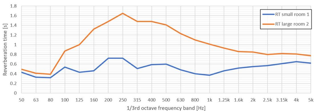
**Figure 16.** Reverberation time measured in mock-up rooms using impulse response.
