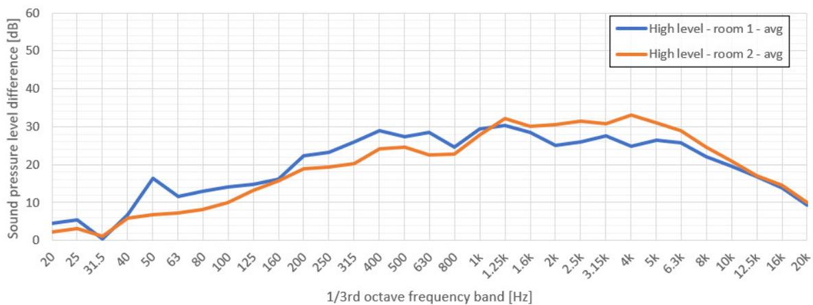
Figure 6. The estimated level difference between the hall and mock-up room during the high-level period. The level difference was obtained from the equivalent sound level in the hall minus the equivalent sound level in the room (1 or 2) recorded during the high-level period (Formula (2)).
