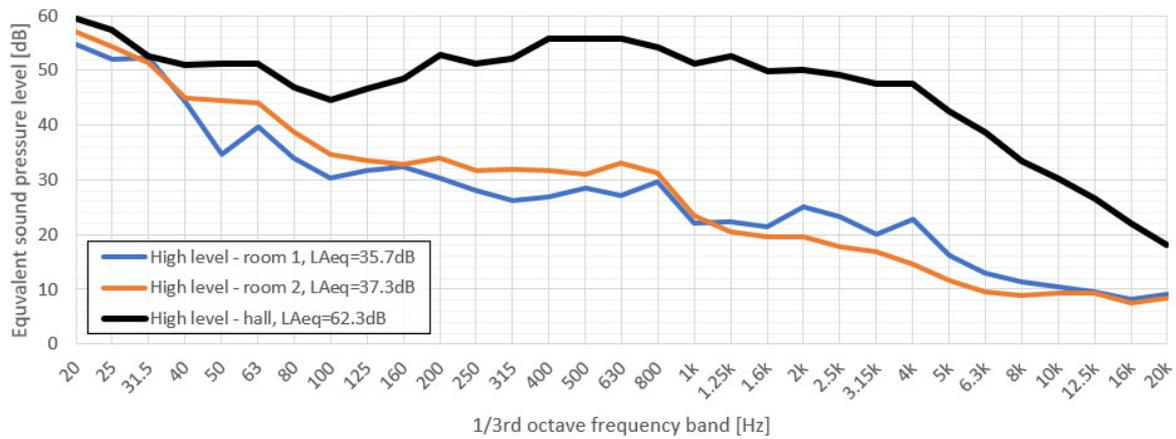
Figure 4. Measured equivalent sound level during the high-level period.
