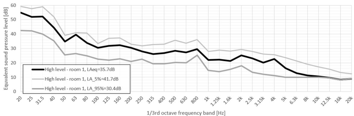
**Figure 9.** Statistical levels of 5% and 95% probability of exceedance for the small mock-up room during the high-level period.
