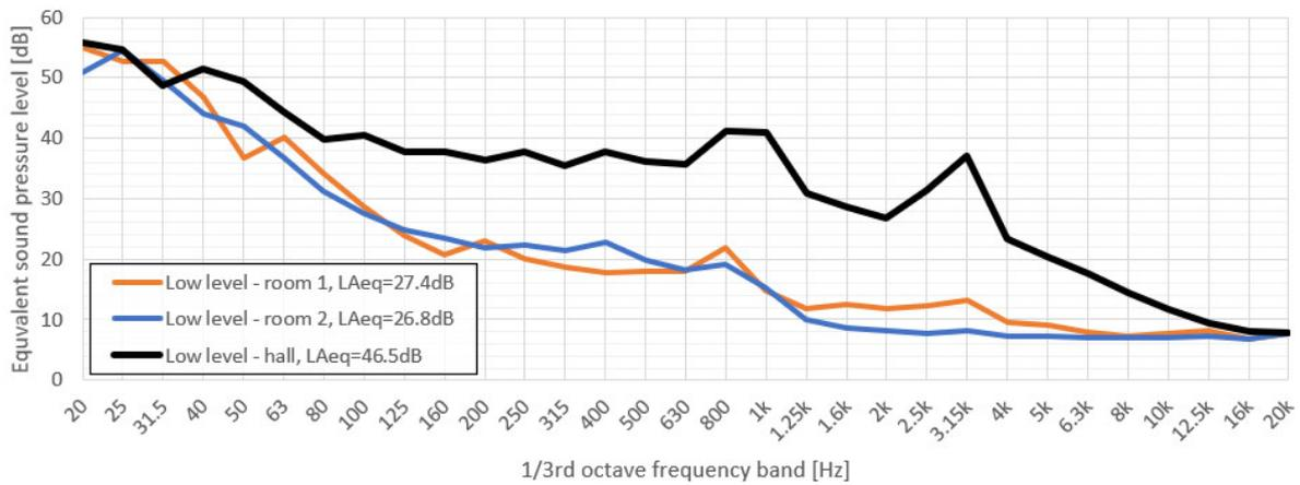
Figure 5. Measured equivalent sound level during the low-level period.
