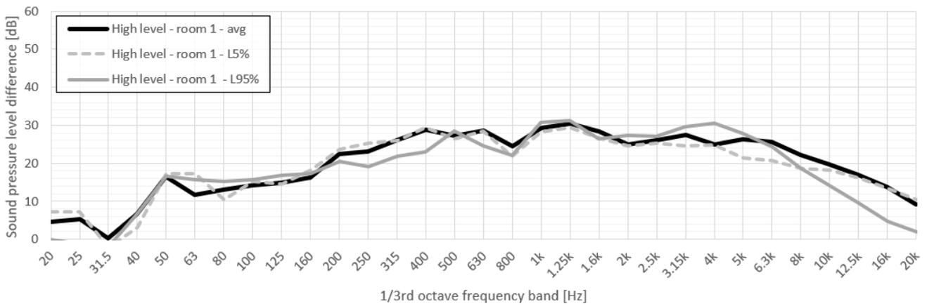
**Figure 10.** The estimated level difference between the hall and small mock-up room 1 during the high-level period with equivalent and statistical levels of L5% and L95% using Formula (2).
