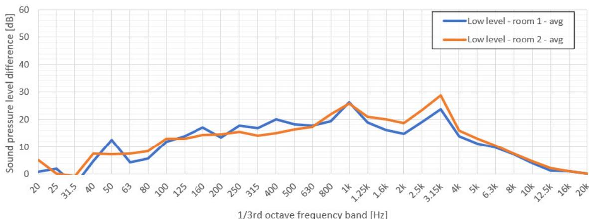
**Figure 7.** The estimated level difference between the hall and mock-up room during the low-level period. The level difference was obtained from the equivalent sound level in the hall minus the equivalent sound level in the room (1 or 2) recorded during the low-level period using Formula (2).
