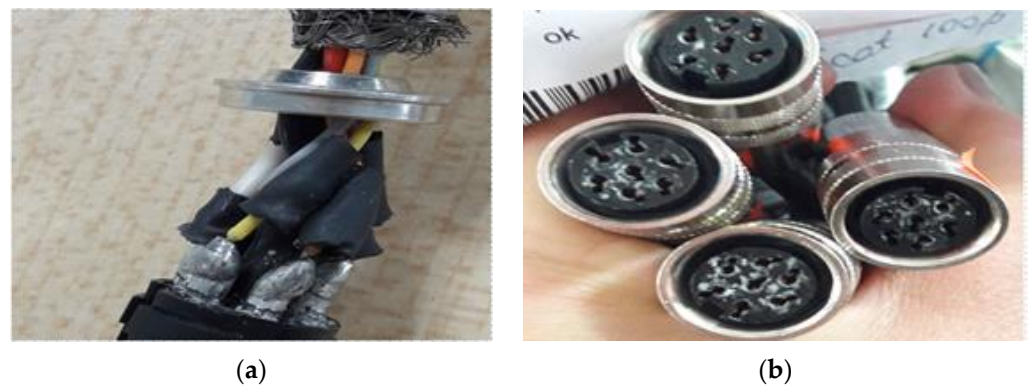
Figure 6. Example of scrap parts in 2Connect Romania: (a) Wire insulation problems; (b) Melted terminal.
