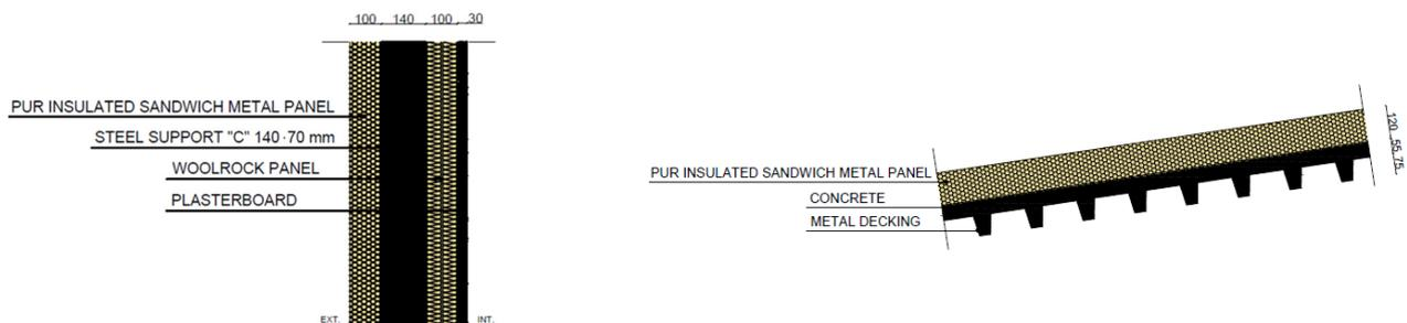
**Figure 2.** Non-structural layout—external walls (left) and roof (right).
