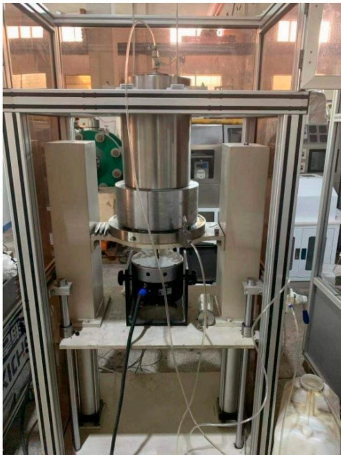
**Figure 2.** Core sample test system.
