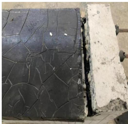
**Figure 8.** Gap between the toughened section and support.
