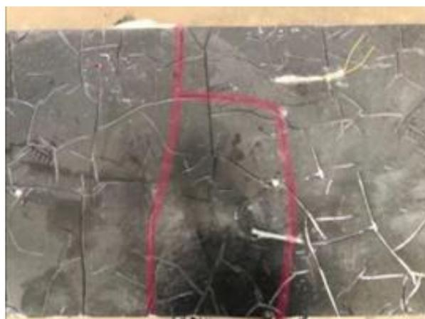
**Figure 5.** Fracture shape of the beam bottom.
