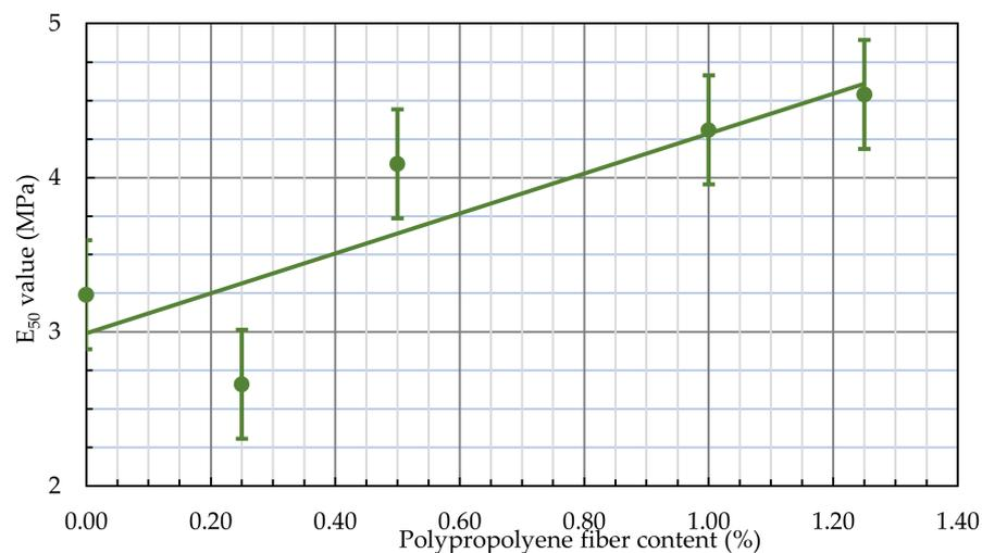
**Figure 19.** E<sub>50</sub> values with different percentages of polypropylene fibers.
