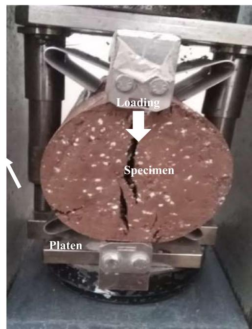
**Figure 6.** Setup for split cylinder testing.
