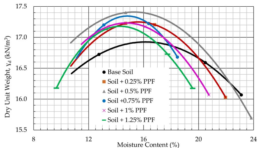
**Figure 10.** Compaction curves for different percentages of PPFs.
