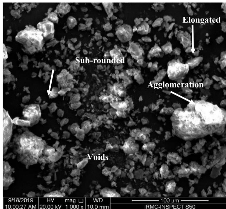
Figure 2. SEM image of the base soil.
