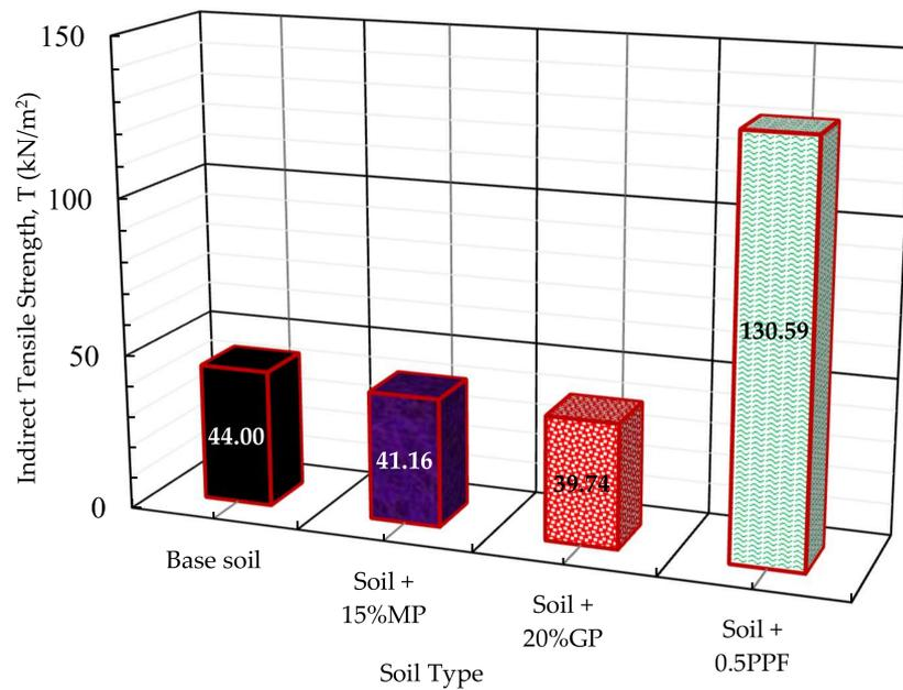
Figure 20. Indirect tensile strength with the optimum percentage of modifiers.
