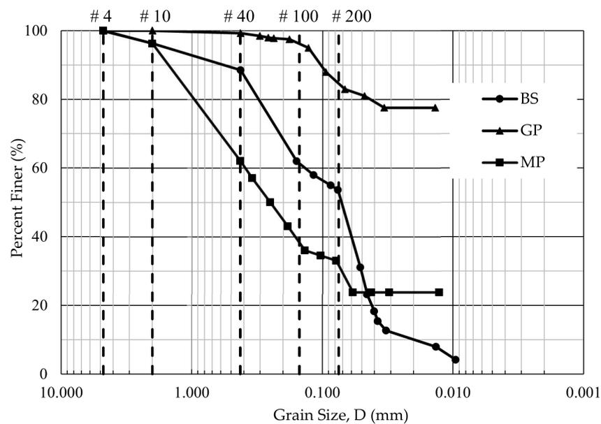
Figure 3. Gradation curves of soil, marble powder, and glass powder.
