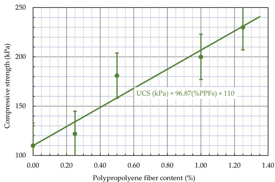
**Figure 17.** Compressive strength variation with different percentages of PPFs.
