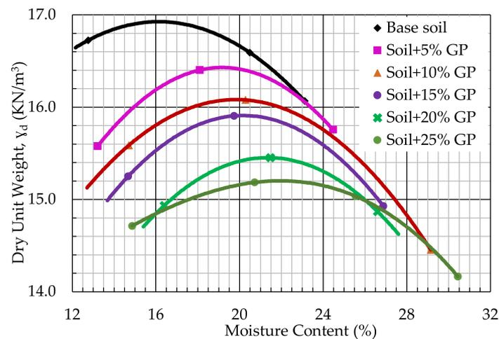
**Figure 8.** Compaction curves with different percentages of GP.
