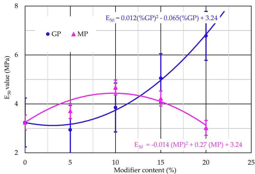
**Figure 18.** E<sub>50</sub> values with different percentages of glass and marble powders.
