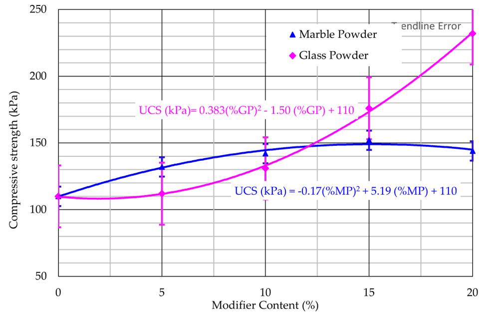
Figure 14. Variation in unconfined compressive strength with modifier content.
