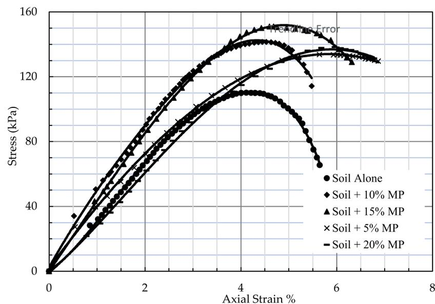
**Figure 12.** Stress strain relationship for different percentages of MP.
