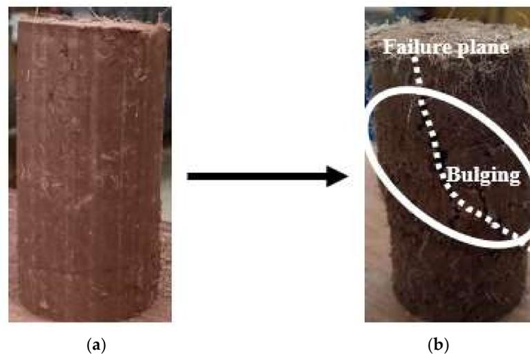
**Figure 16.** Fiber reinforced soil sample (a) before and (b) after UCS test.
