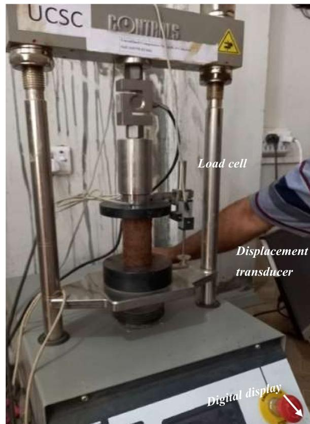
**Figure 5.** Test setup for the unconfined compressive strength.
