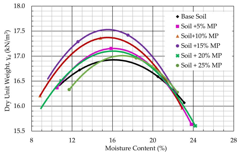
**Figure 7.** Compaction curves with different percentages of MP.
