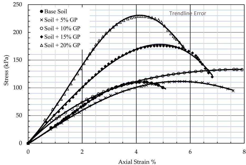
Figure 13. Stress-strain relationship for varying content of GP.
