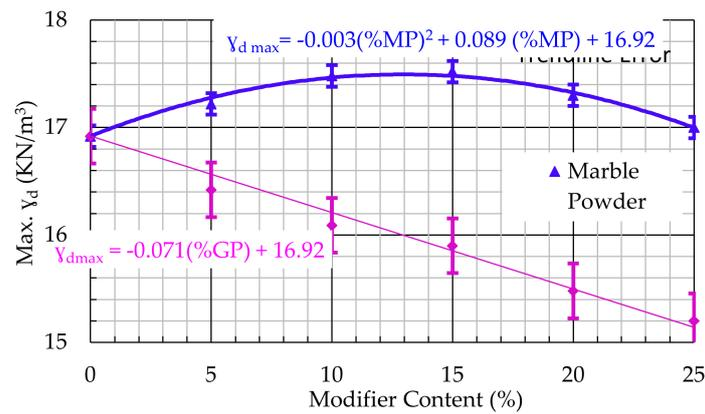
**Figure 9.** Relationship between modifier content and maximum dry density.
