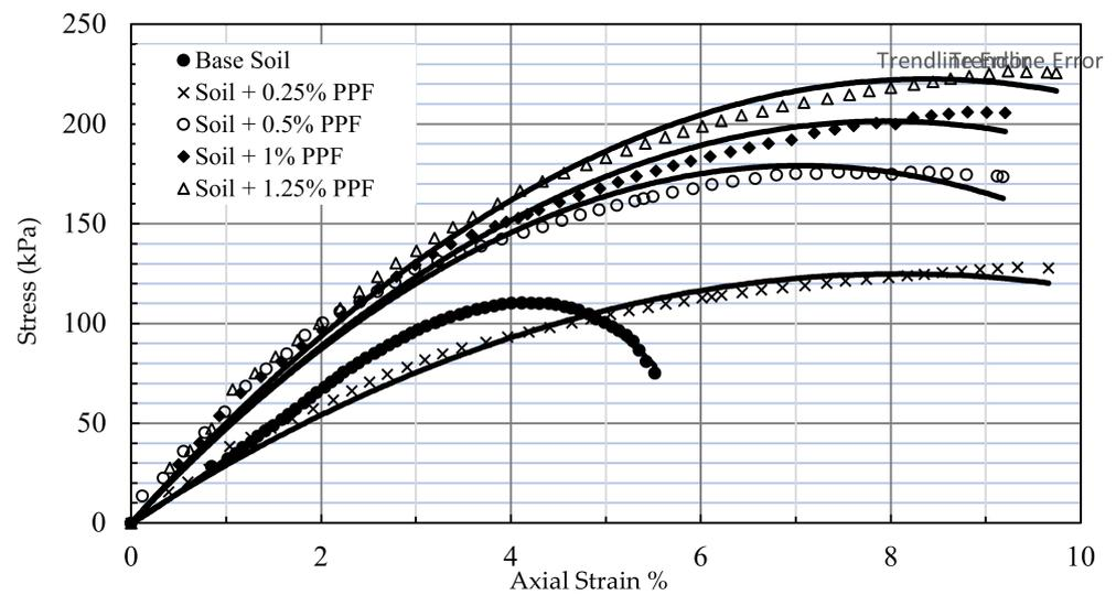
**Figure 15.** Stress-strain plot for different percentages of PPFs.
