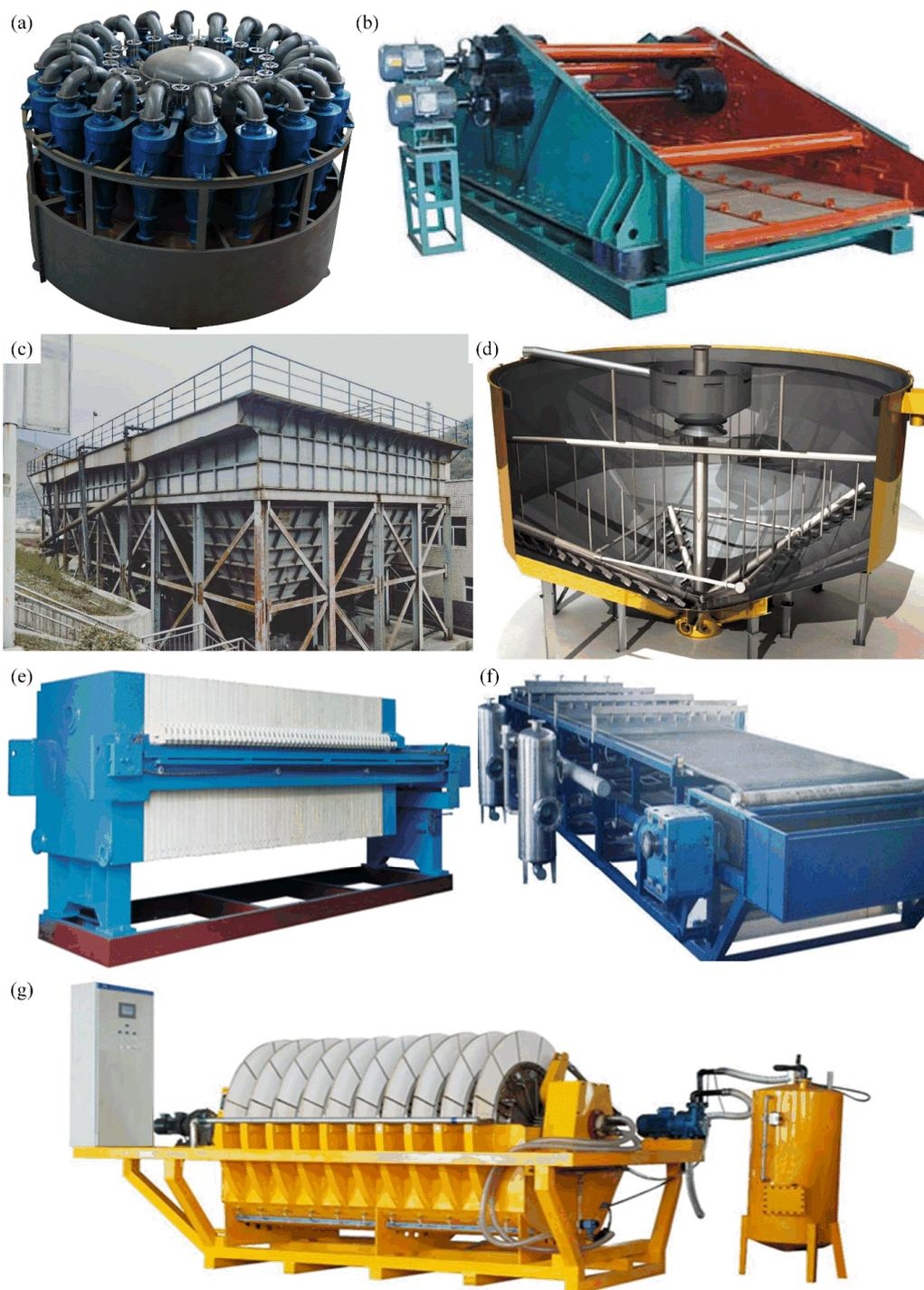
**Figure 7.** Tailings thickener dehydration equipment: (a) hydrocyclone; (b) high frequency vibration dehydration sieve; (c) inclined plate thickener; (d) deep cone thickener; (e) plate and frame filter press;
