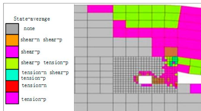
**Figure 8.** Development characteristics of plastic zone of surrounding rock during roadway driving.
