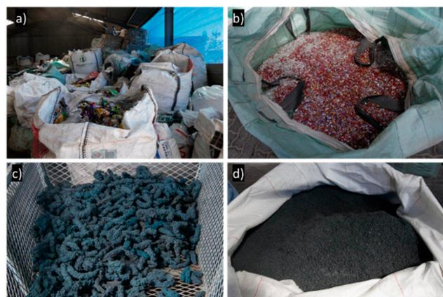
**Figure 4.** Production process for Resin8, (a) plastic wastes collected, (b) plastic flakes, (c) heat extruded plastic before grinding, (d) Resin8 plastic aggregate.
