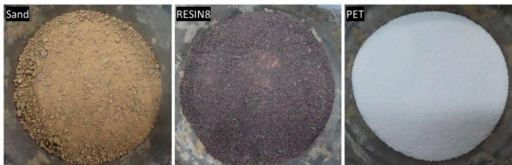
Figure 2. Fine aggregates used for mixing.
