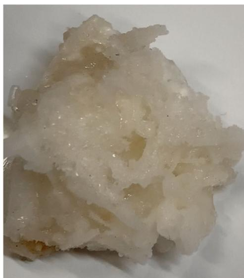
**Figure 12.** Particulate of  $\text{CO}_2$  hydrate extracted from the reactors; the growth of crystals caused the formation of numerous macro cavities, where the high  $\text{NH}_4^+$  concentration-liquid phase was physically captured.
