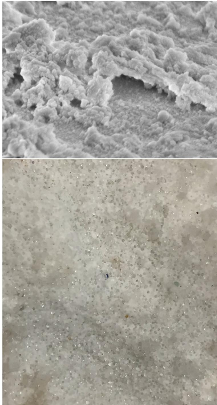
**Figure 4.** Picture above: scanning microscope high-resolution image of a single grain (scale: 200 nm). Picture below: the porous sediment extracted from the reactor after the formation of CO<sub>2</sub> hydrates. The clathrate structures formed between grains and cemented the whole sediment.
