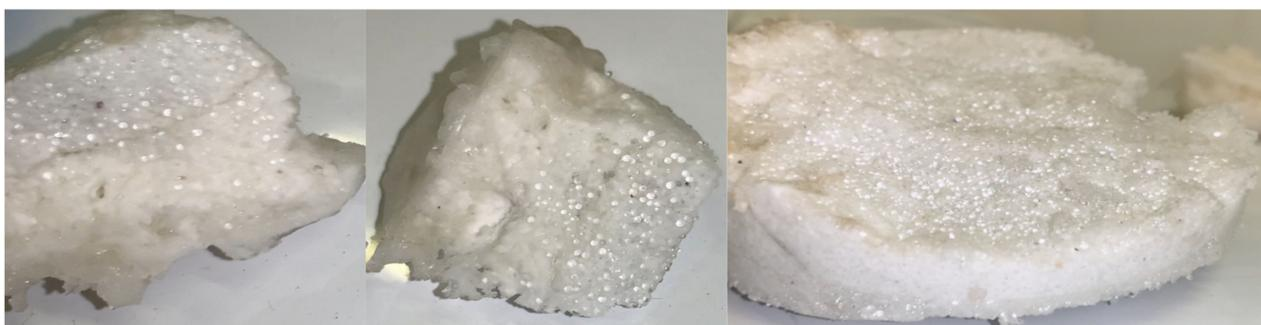
**Figure 11.** Pictures of hydrate samples extracted from the reactors.
