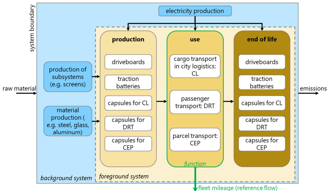
**Figure 3.** Product system of the U-Shift vehicle fleet for the defined use case (CL—city logistics; CEP—parcel delivery services consisting of courier, express, parcel delivery; DRT—demand responsive transport for public transport).
