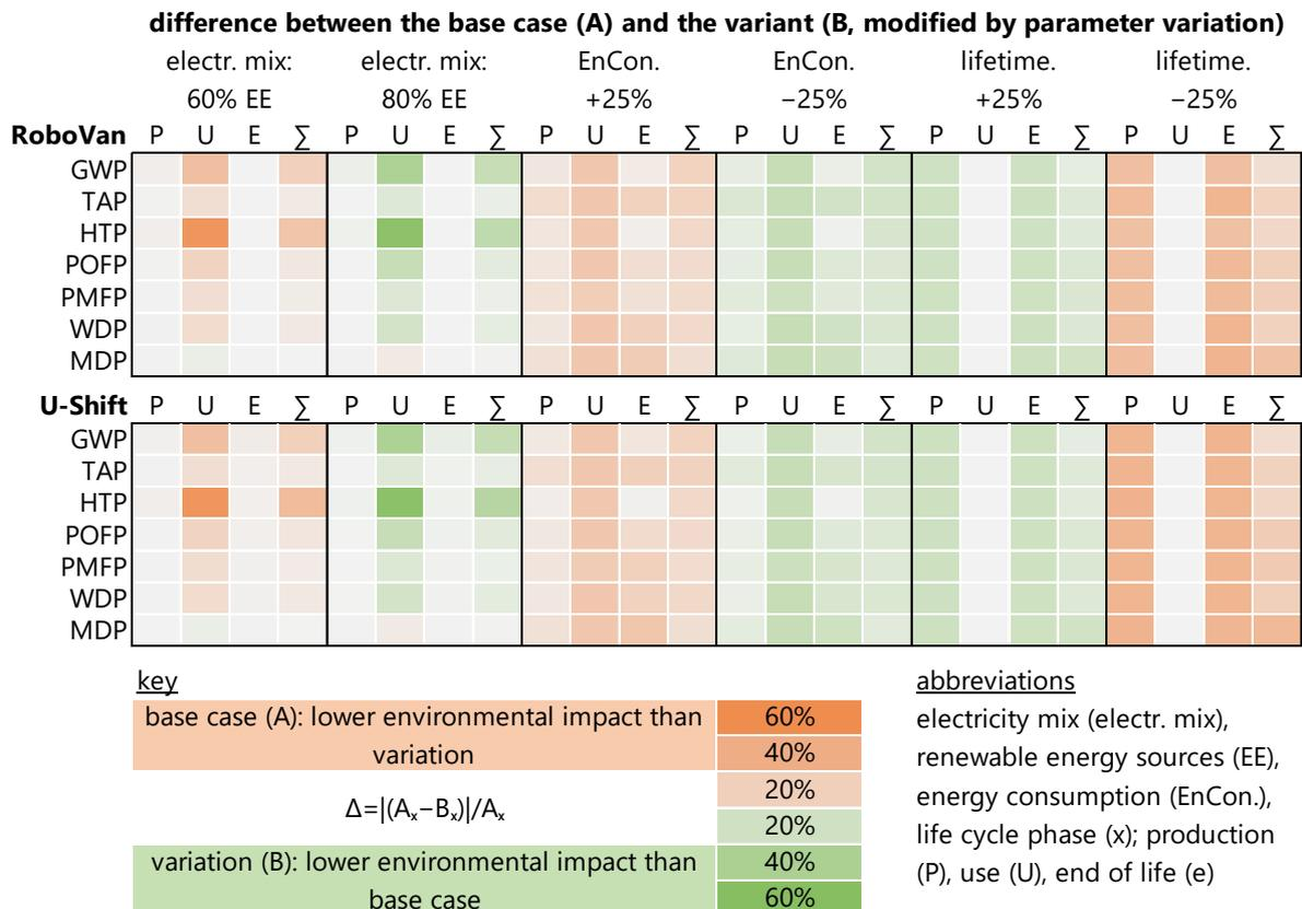
**Figure 6.** Vehicle-specific sensitivity analyses by varying different parameters (impact categories are defined in Table 5).
