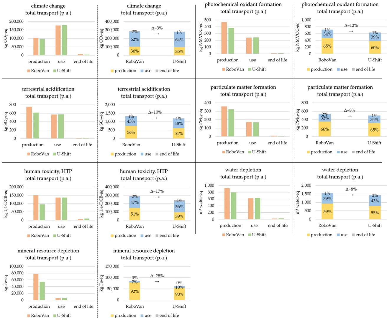
**Figure 5.** Detailed analysis of selected impact categories comparing the RoboVan and the U-Shift fleet.
