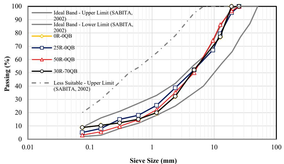
**Figure 2.** Gradation curves for selected EAM blends [5].
