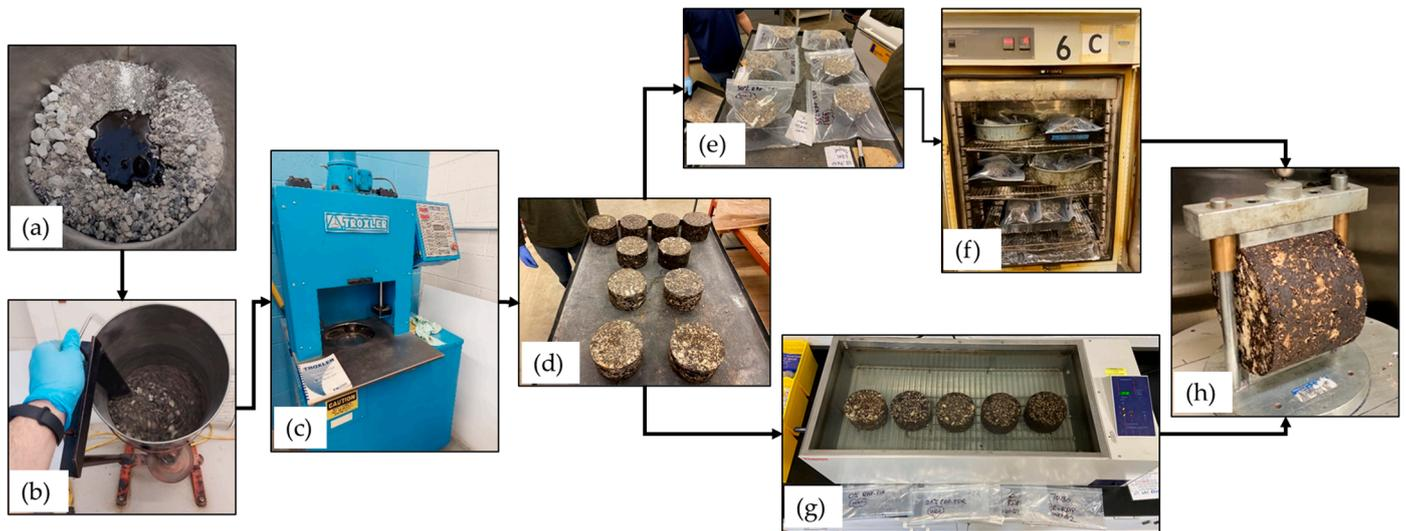
**Figure 4.** ITS specimen preparation and testing: (a) emulsion in aggregate blend, (b) drum mixing, (c) SGC, (d) air drying for 24 h, (e) sealed specimens, (f) oven draft curing at 40 °C for 48 h, (g) wet curing in water bath at 25 °C for 24 h, and (h) specimen in ITS testing rig.
