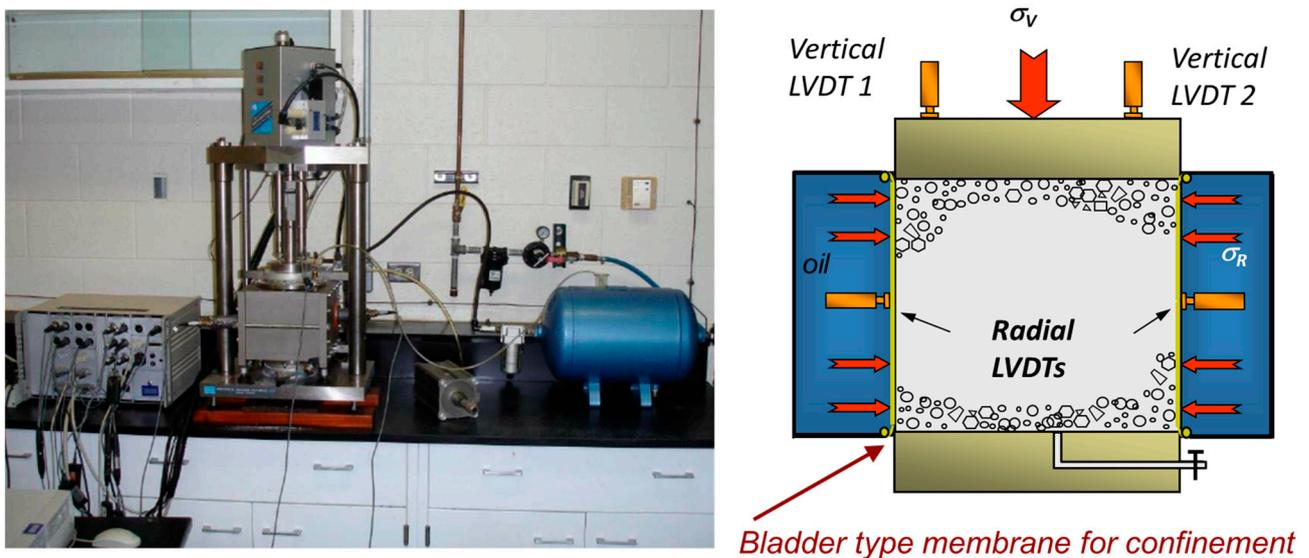
**Figure 5.** The University of Illinois FastCell (UI-FastCell) device.
