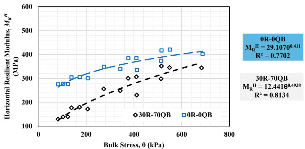
Figure 11. Horizontal resilient modulus ( $M_R^H$ ) for 30R-70QB.
