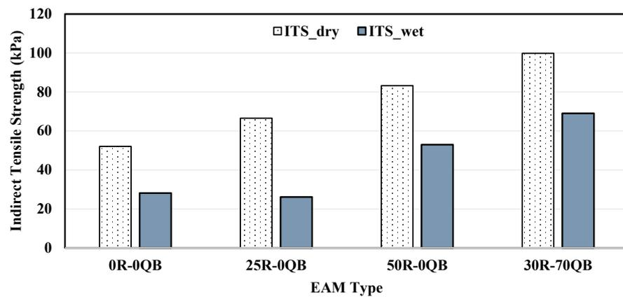
Figure 6. Effect of blend constituent composition on the Indirect Tensile Strength (ITS) of the EAMs.
