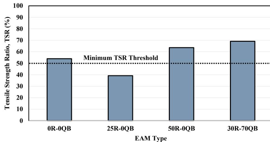
Figure 7. Effect of blend composition on the Tensile Strength Ratio (TSR) of the EAMs.
