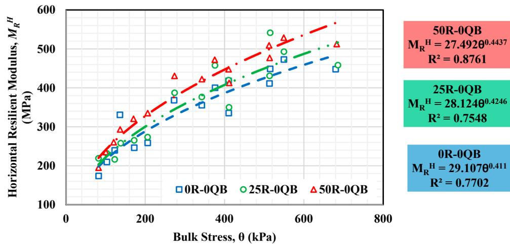
Figure 10. Effect of variation in FRAP on horizontal resilient modulus ( $M_R^H$ ).
