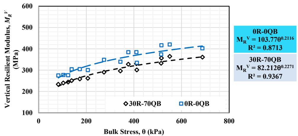
Figure 9. Vertical resilient modulus ( $M_R^V$ ) for 30R-70QB.
