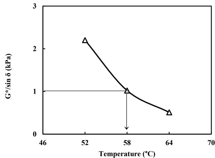
**Figure 3.** Performance grade of asphalt binder extracted from HFE-300 anionic emulsion.
