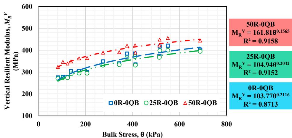
Figure 8. Effect of variation in FRAP on vertical resilient modulus ( $M_R^V$ ).
