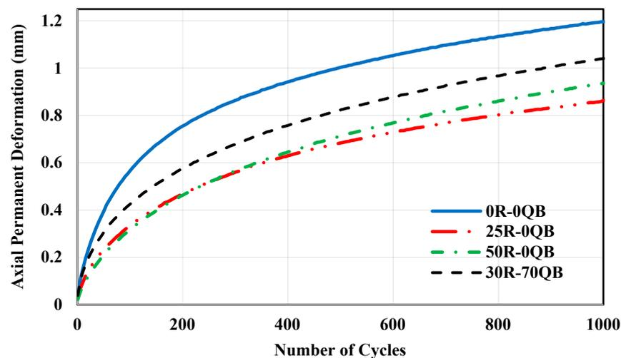
Figure 13. Effect of EAM blend composition on permanent deformation.
