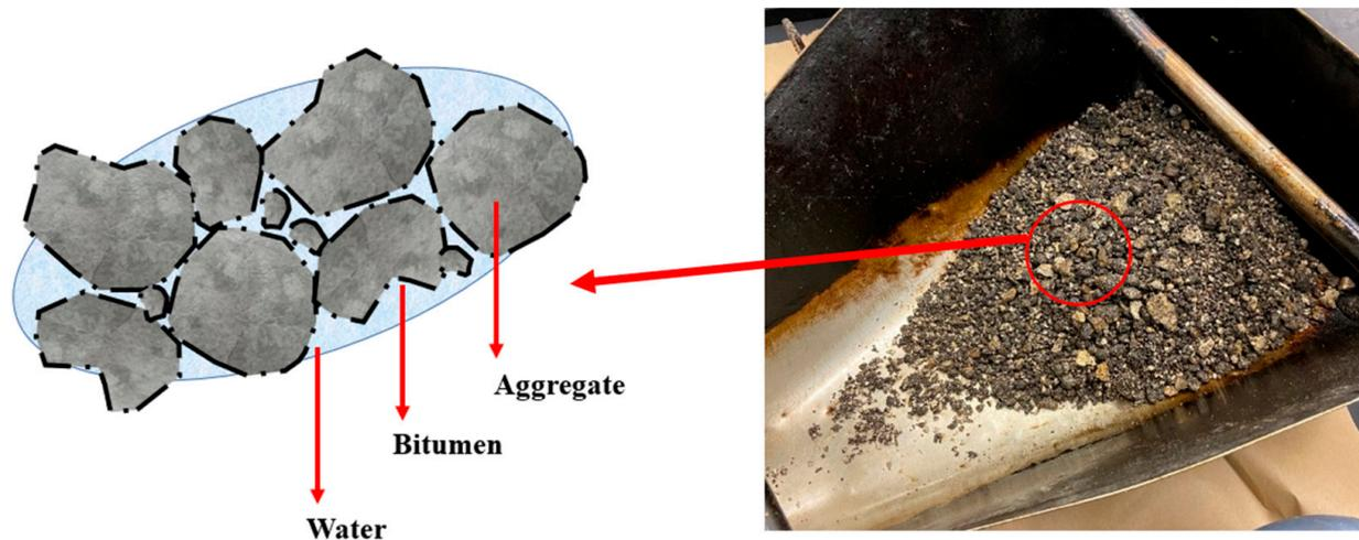
Figure 1. Composition of a typical EAM.
