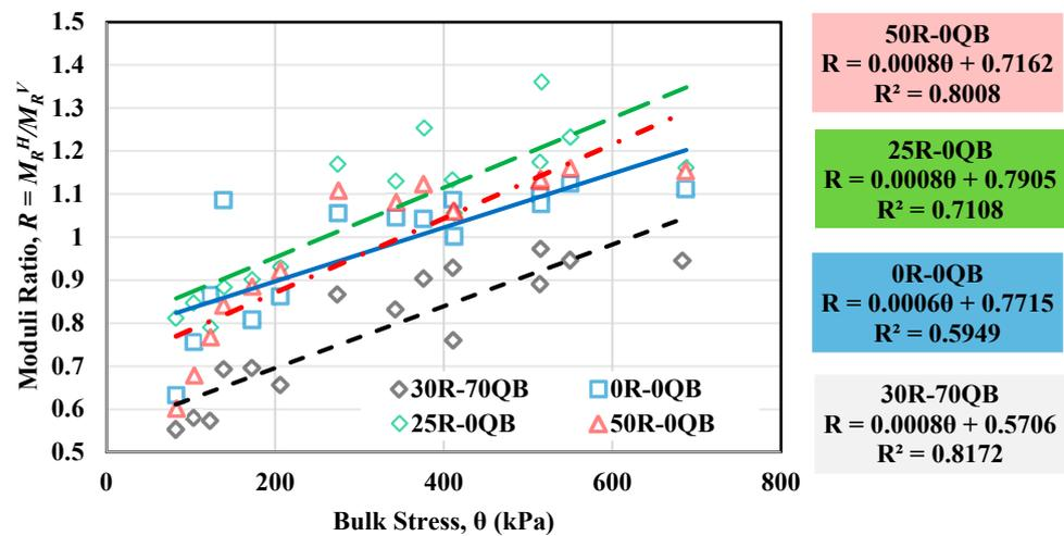
Figure 12. Effect of EAM blend composition on  $M_R^H/M_R^V$ .
