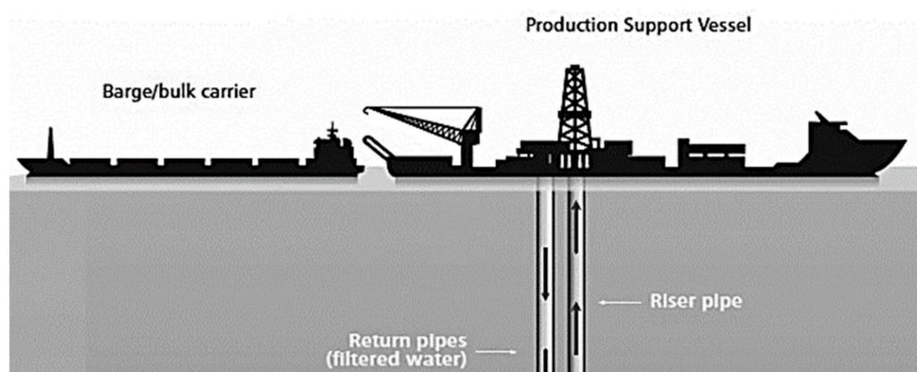
**Figure 2.** Nodules recovery and transportation process [24].
