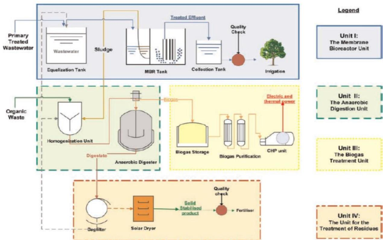
Figure 1. Simplified flow chart of the integrated MBR-AD system.
