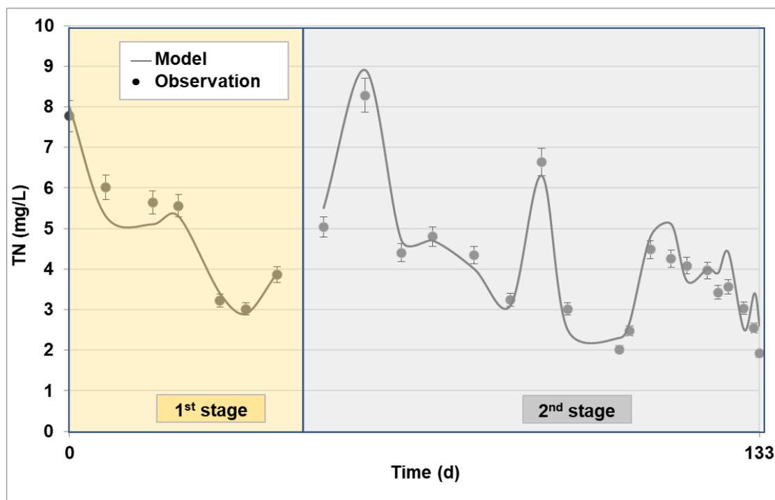
**Figure 4.** Measurements and simulated values of TN concentration derived from the calibration of the model.
