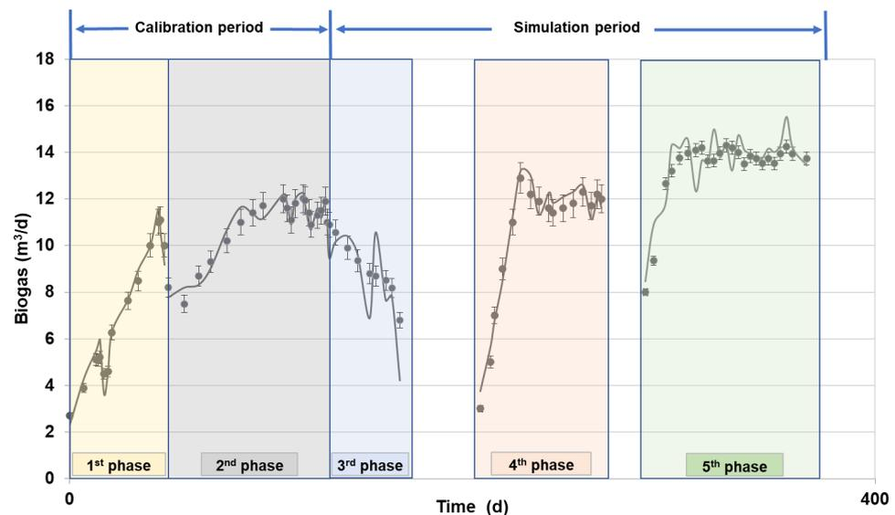
**Figure 7.** Experimental values of biogas production for all phases, as well as the calibrated (1st and 2nd phases) and simulated (3rd to 5th phases) values.
