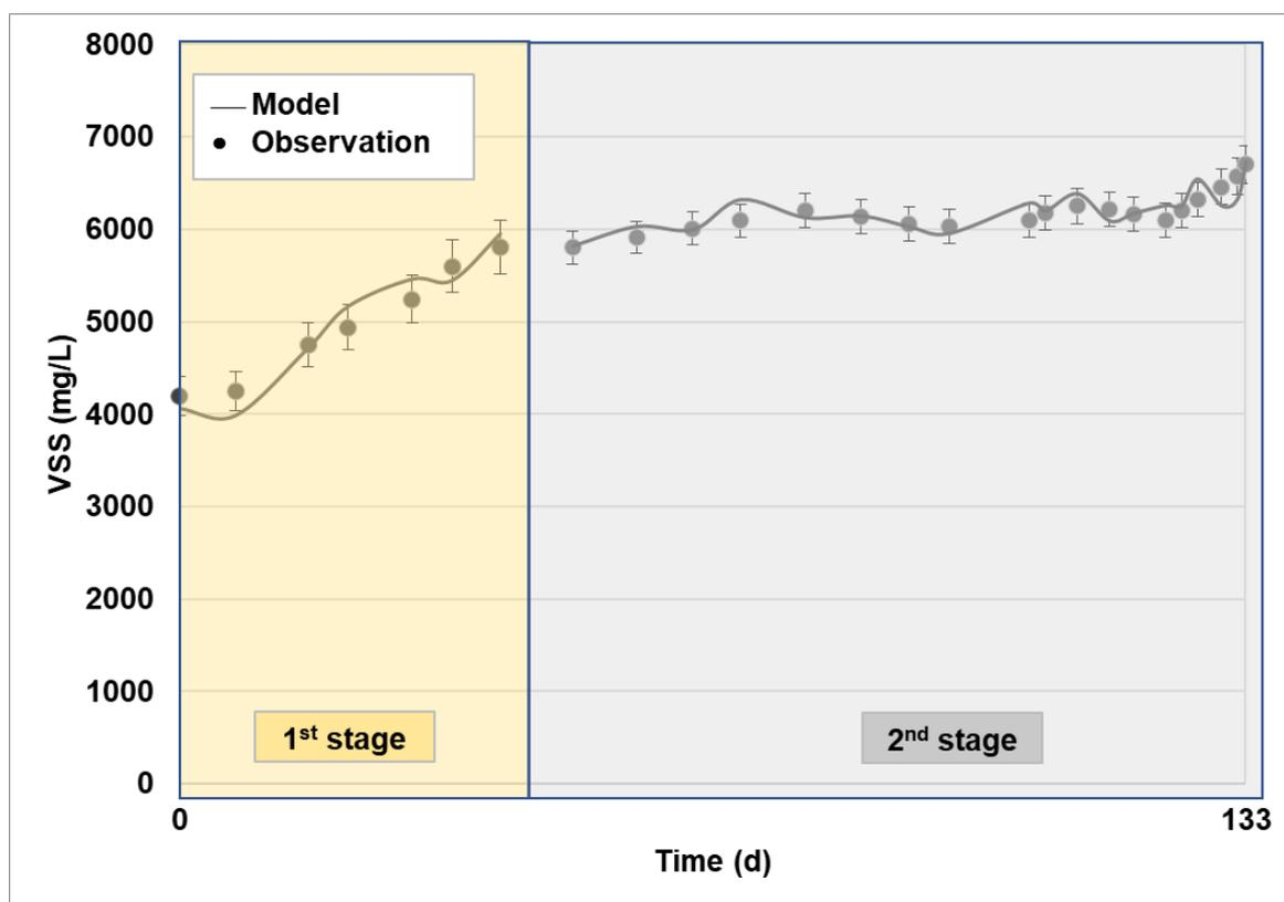
**Figure 3.** Measurements and simulated values of VSS concentration derived from the calibration of the model.
