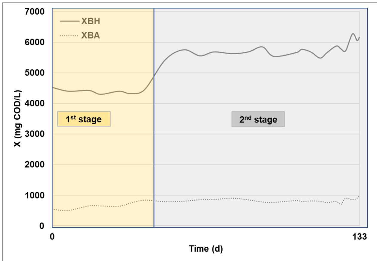
**Figure 5.** Active biomass concentration: heterotrophic  $X_{BH}$  and autotrophic  $X_{BA}$  as predicted from the model.
