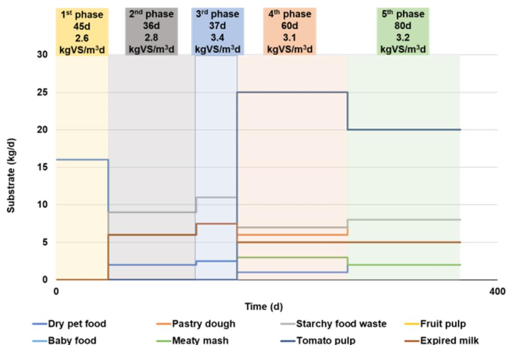
**Figure 2.** Feeding schedule and OLR of each experimental phase during the anaerobic digestion process.
