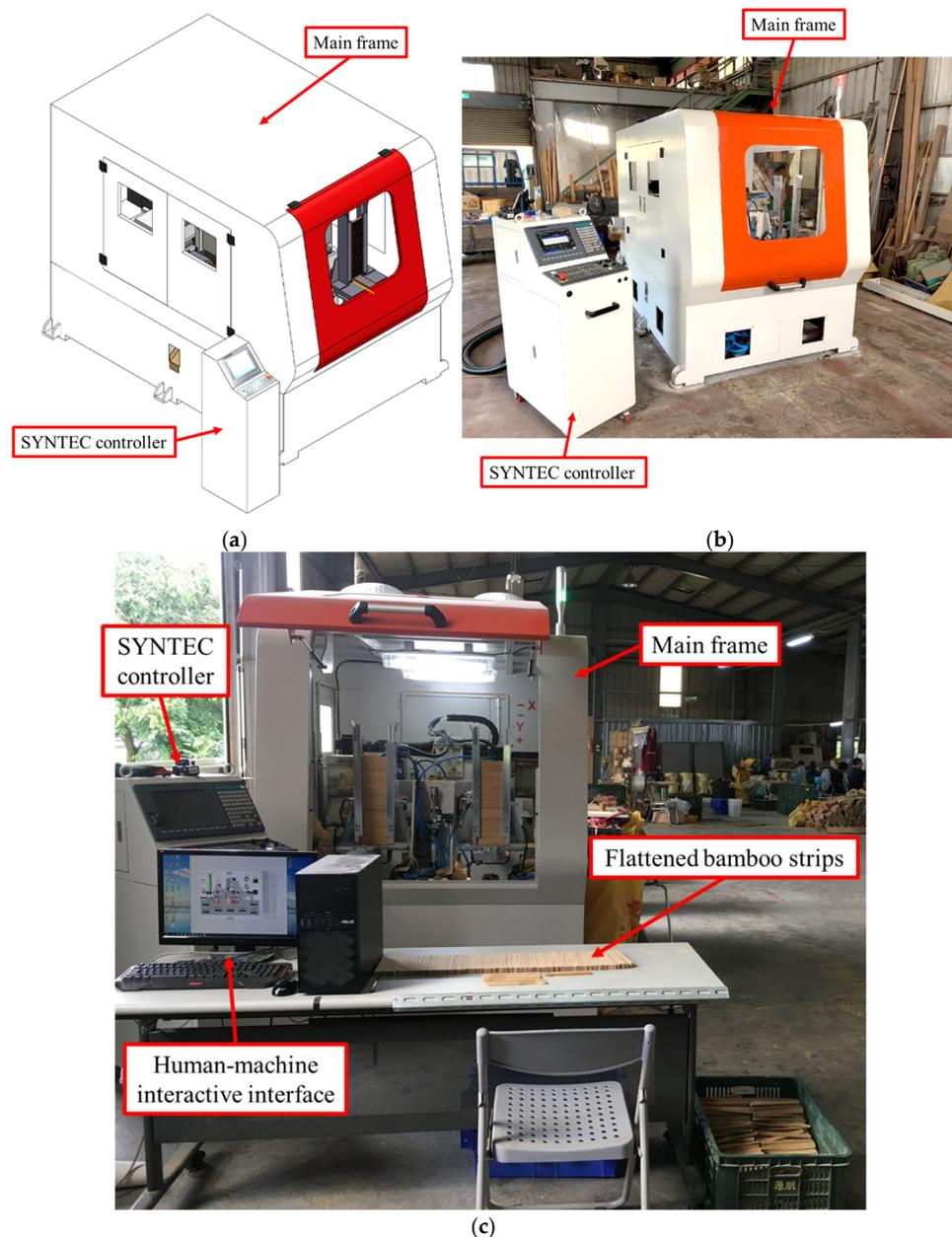
**Figure 17.** The fabricated bamboo toothbrush handle machine: (a) schematic diagram, (b) actual machine, and (c) entire structure.
