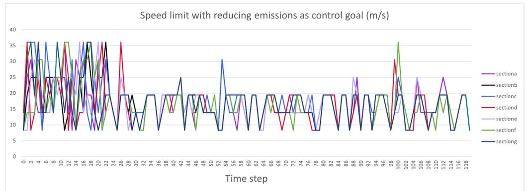
Figure 11. The speed limit of different road sections with reducing emissions as a control goal.
