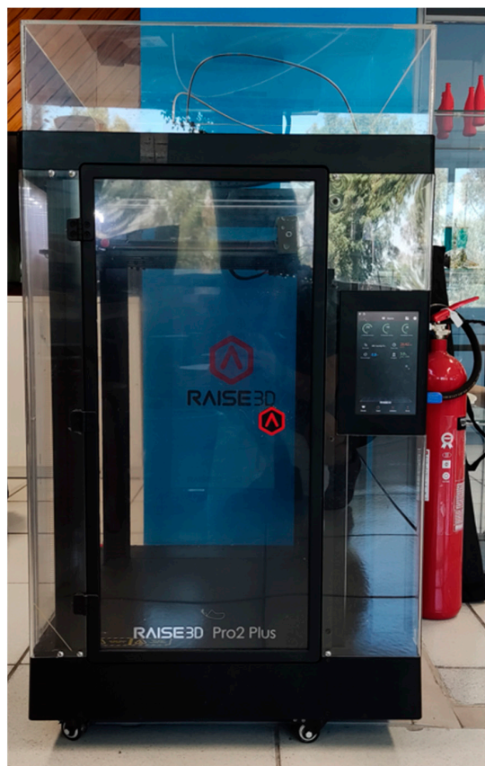
Figure 5. Raise3D™ Pro2™ Plus 3D printer used to fabricate the scaled statue replicas.
