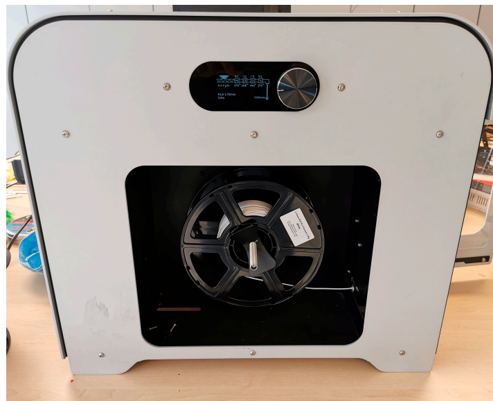
Figure 7. 3D Evo Composer filament maker equipment that was used in this case.
