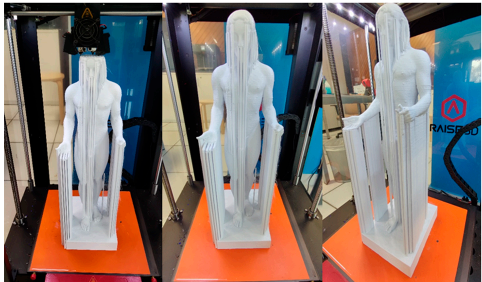
Figure 14. Apollo of Piraeus statue replica upon the completion of the 3D printing process.
