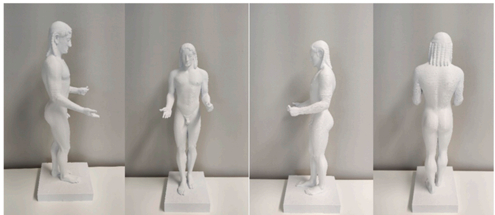
Figure 15. Apollo of Piraeus statue replica upon the completion of the 3D printing process and support structures removal.
