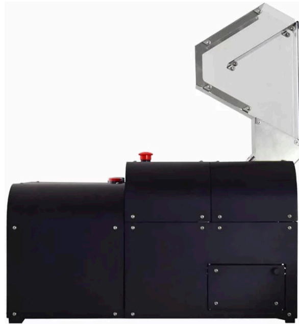
Figure 6. 3D Evo SHR3D material shredding equipment that was used in this case.
