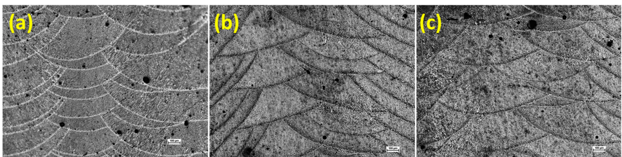
Figure 6. Melt pool profile and depth at different laser powers: (a) 800–600 w, (b) 1100–670 w, (c) 1000–750 w.
