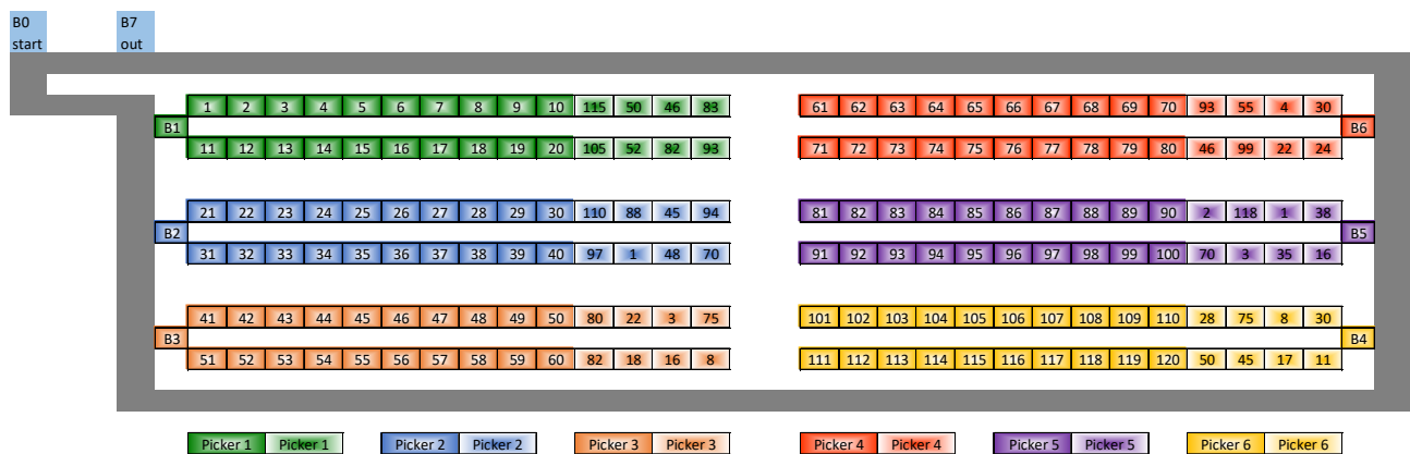
Figure 2. Distribution center layout; each employee is responsible for one buffer: B0 and B7 are containers in and out buffers; order picking is realized in buffers from B1 to B6; darker colors mean places with products exclusive to that buffer; lighter colors mean places of products that can also be found on other buffers.
