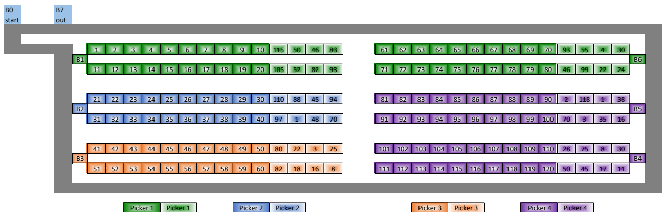
Figure 3. Distribution center layout; one employee is responsible for more than one buffer: B0 and B7 are containers in and out buffers; order picking is realized in buffers from B1 to B6; darker colors mean places with products exclusive to that buffer; lighter colors mean places of products that can also be found on other buffers.
