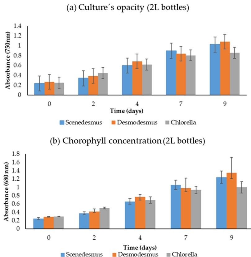
**Figure 5.** Measurements in 2 L experiments with wastewater: (a) absorbance at  $OD_{750}$  for opacity evaluation, (b) absorbance measurements at  $OD_{680}$  for chlorophyll content evaluation.
