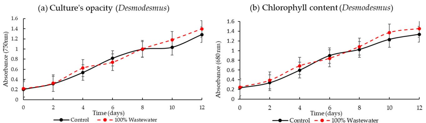
**Figure 6.** Measurements in 2 L experiments with *Desmodesmus* sp. growth with wastewater and the control (without wastewater): (a) absorbance at OD<sub>750</sub> for opacity evaluation, (b) absorbance measurements at OD<sub>680</sub> for chlorophyll content evaluation.
