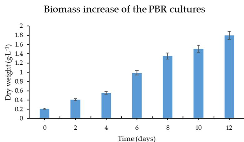
Figure 8. Dry weight biomass measurements during closed-type PBR culturing.
