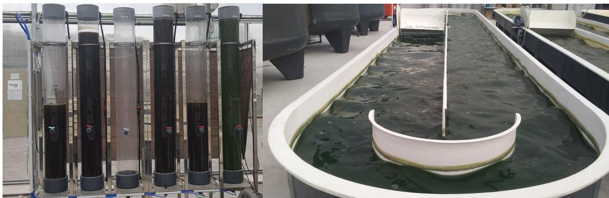
**Figure 3.** Pilot-scale microalgae cultivation systems at NEOALGAE: vertical closed PBRs (left), open raceways (right).
