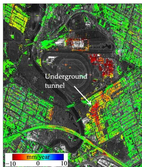
**Figure 17.** Estimated ground deformation rate with CSK dataset in LOS direction relating to the underground construction.
