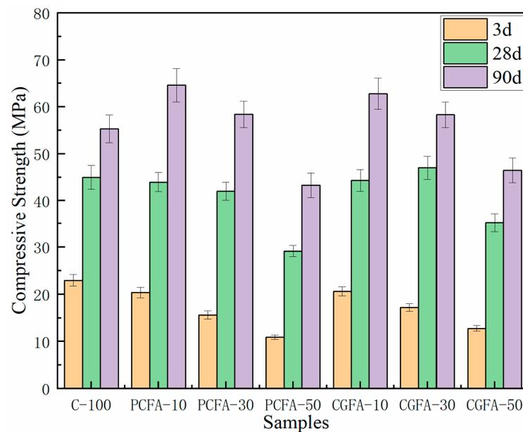
**Figure 4.** The compressive strength of different cement mortar.
