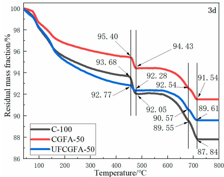
**Figure 10.** Thermogravimetric analysis of cement hydration sample containing CGFA and UGCGFA after 3 days of hydration.
