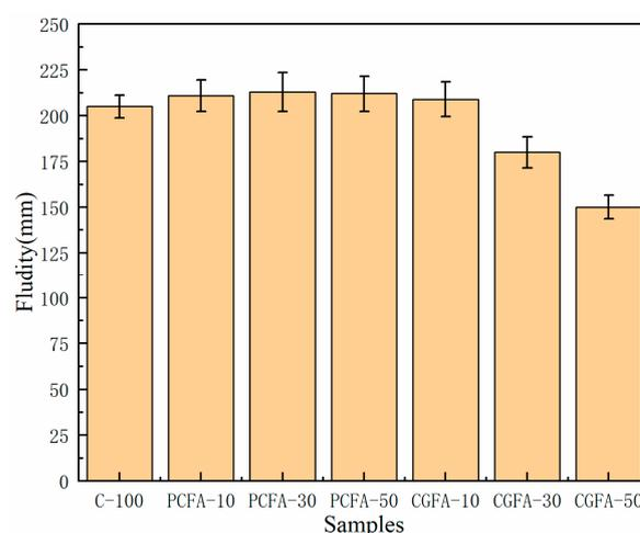
**Figure 3.** The fluidity results of cement mortar containing PCFA or CGFA.
