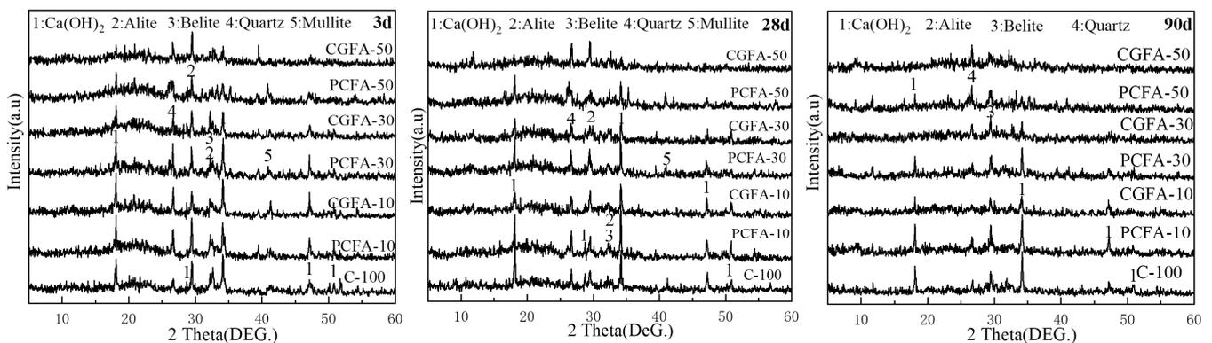
**Figure 5.** XRD patterns of 3 d, 28 d, and 90 d hydration products of PCFA or CGFA-cement.
