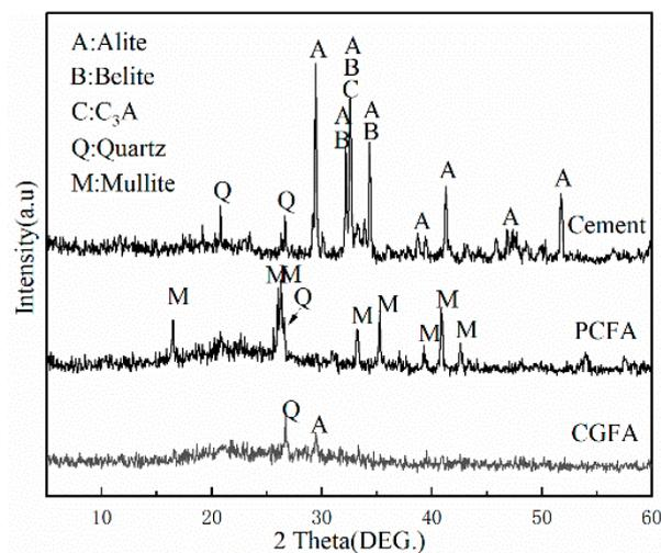
**Figure 1.** XRD spectra of CGFA, PCFA, and cement.
