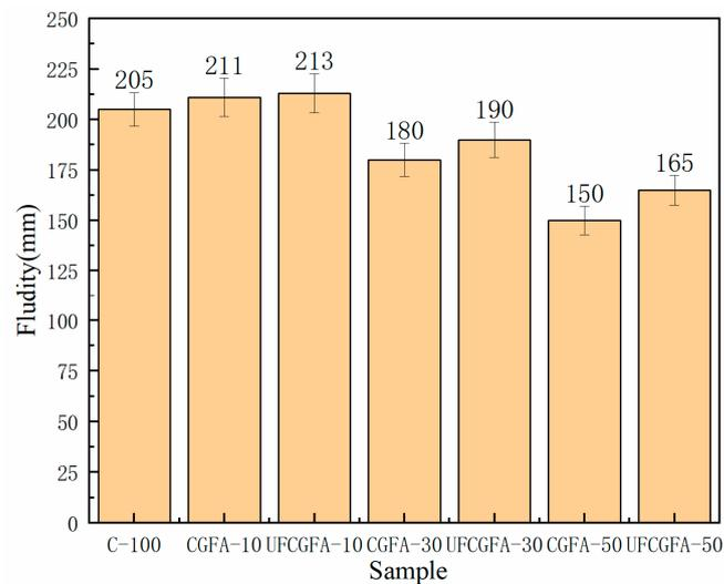
**Figure 7.** Fluidity of CGFA or UFCGFA-cement mortar.
