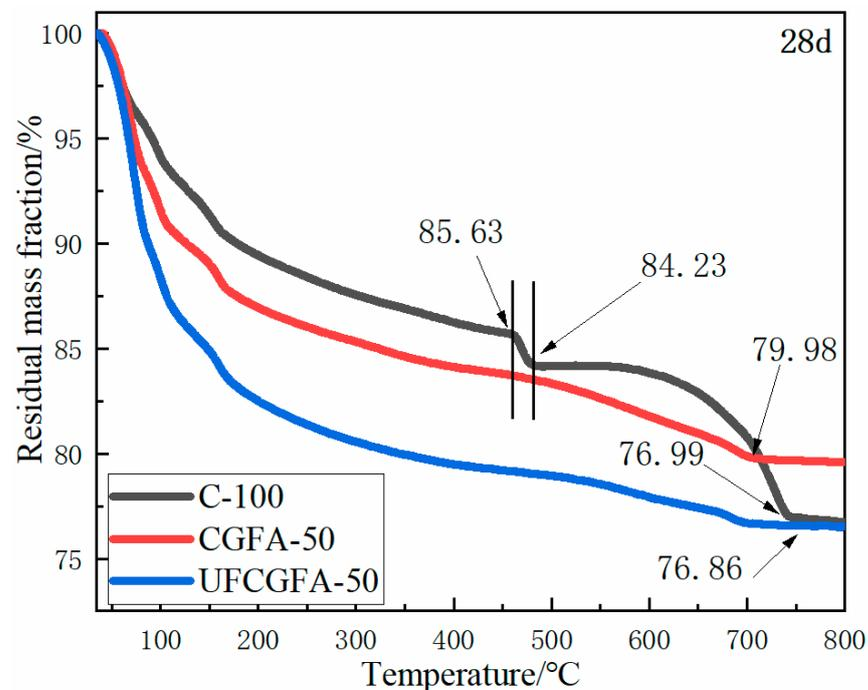
**Figure 11.** Thermogravimetric analysis of cement hydration sample containing CGFA and UGCGFA after 28 days of hydration.
