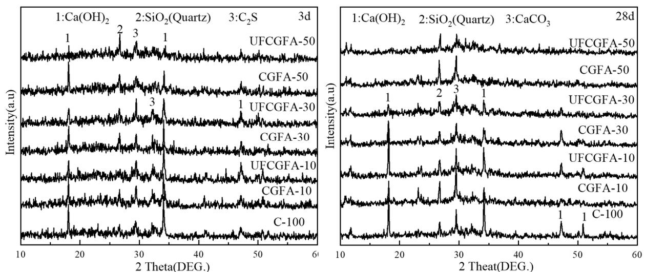
Figure 9. XRD diffraction spectra of cement mortar with CGFA or UFCGFA.
