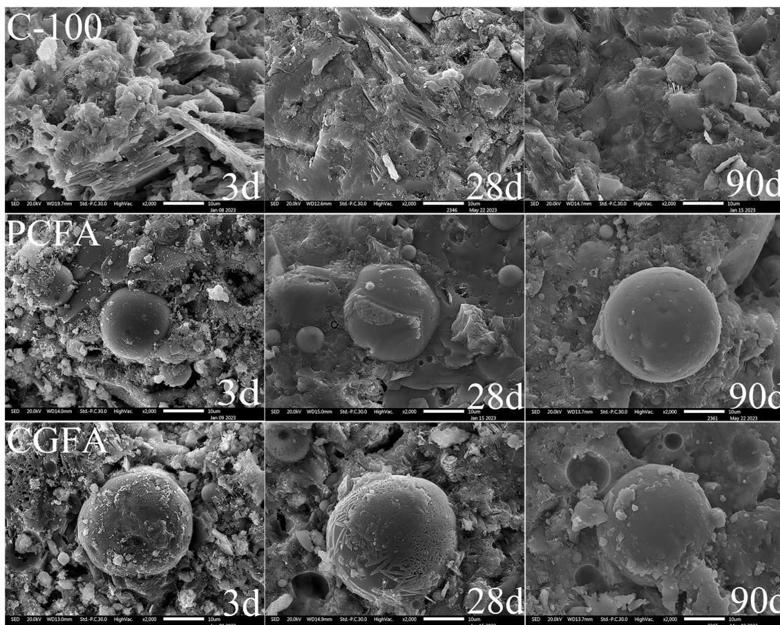
**Figure 6.** The microstructure of cement hydration sample containing PCFA and CGFA.
