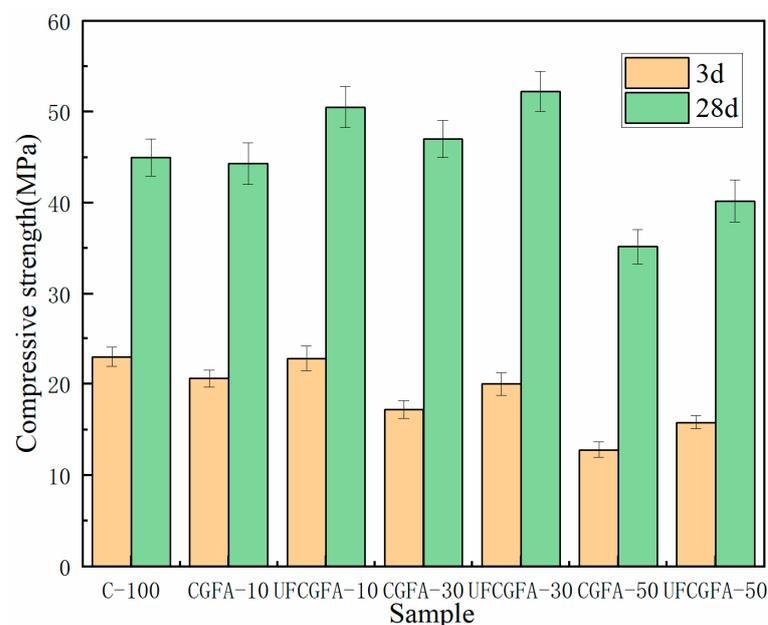
**Figure 8.** The compressive strength of cement mortar with CGFA or UFCGFA.
