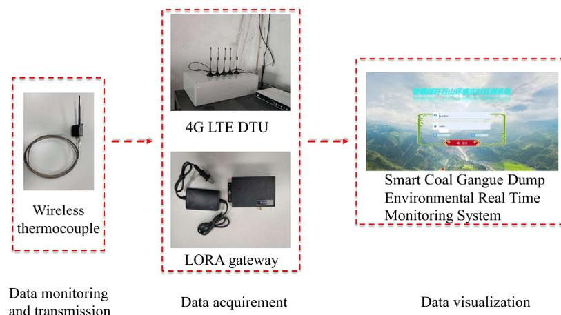
**Figure 7.** Smart dynamic cloud monitoring system.
