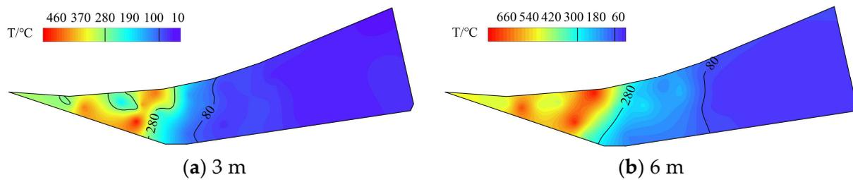
**Figure 8.** Initial temperature distribution of different depths of the coal gangue dump.
