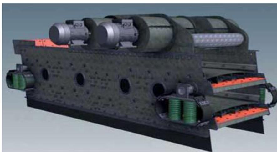
**Figure 7.** PC-model of the sifter. Source: Own study.
