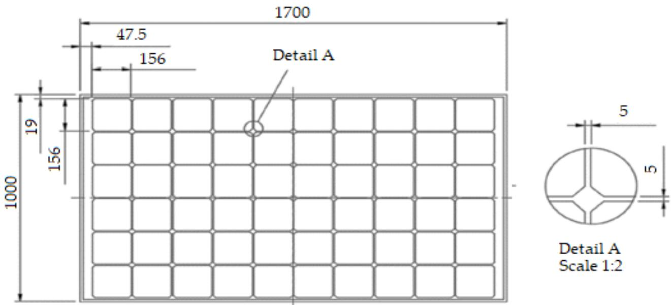
**Figure 1.** Sketch of a standard PV panel. Source: Own study.
