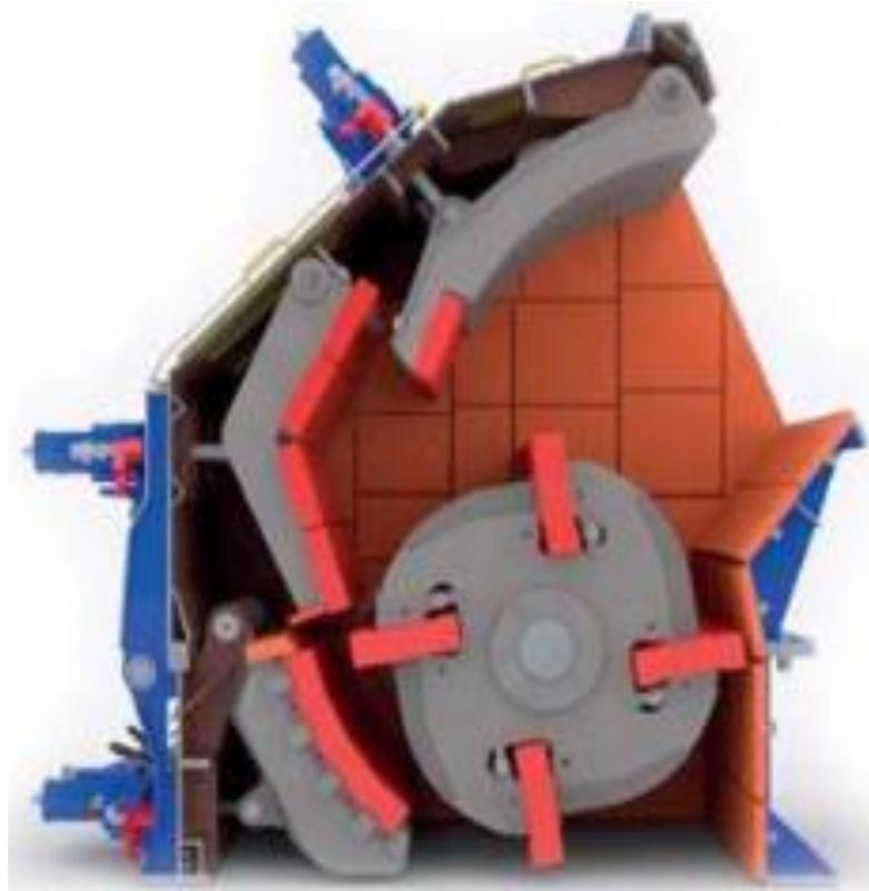
**Figure 6.** Cross-section of the primary crusher for the version with 3 crushing plates. Source: Own study.
