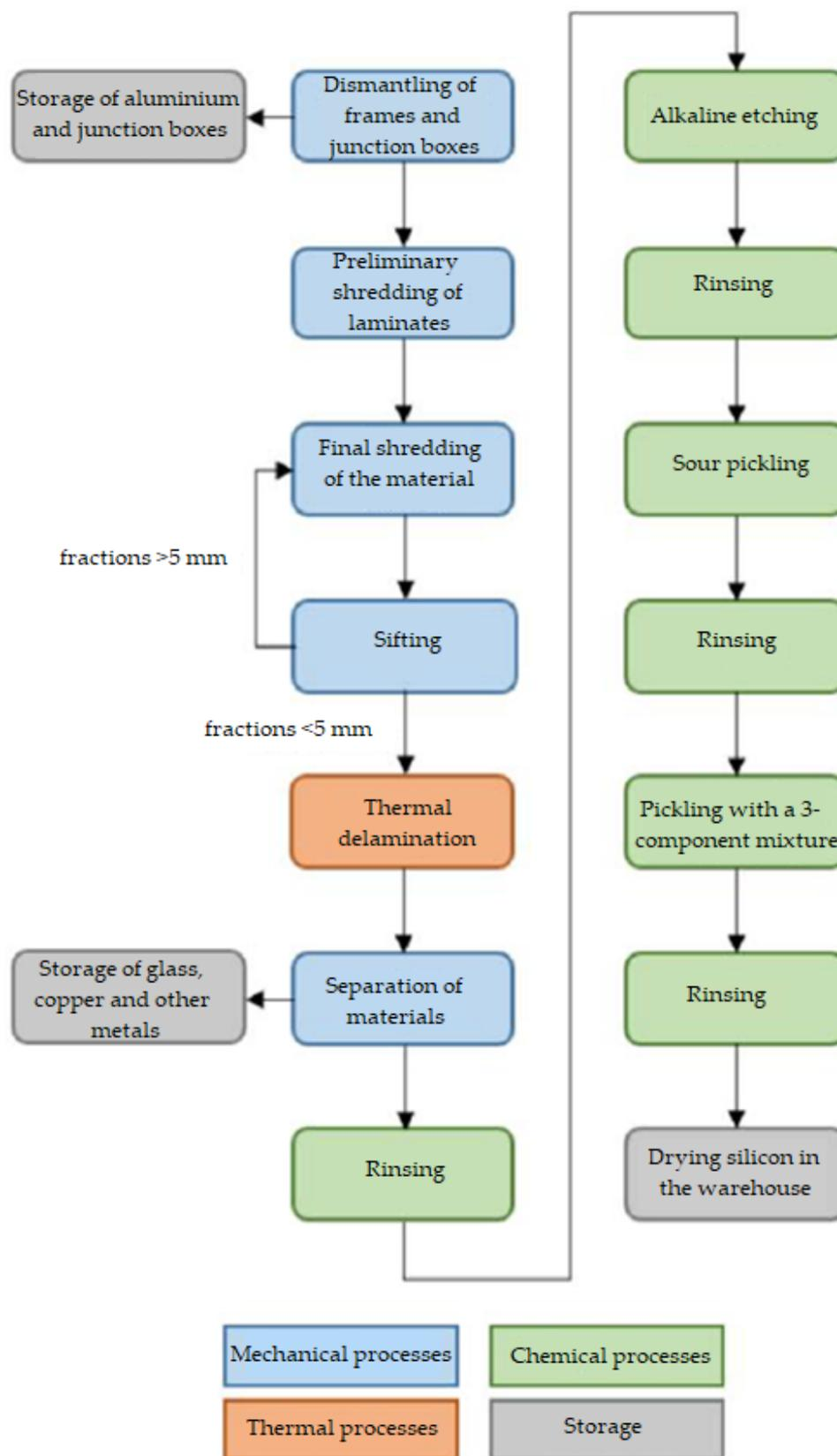
**Figure 2.** Block diagram of the process of recycling photovoltaic panels, taking into account the type of process. Source: Own study.
