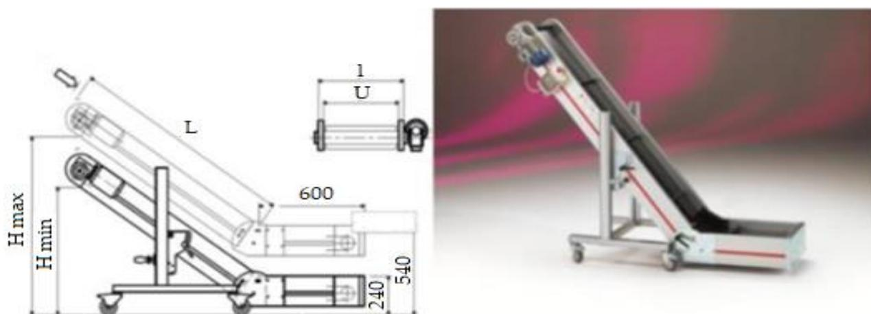
Figure 9. Example of an articulated belt conveyor. Source: Own study.
