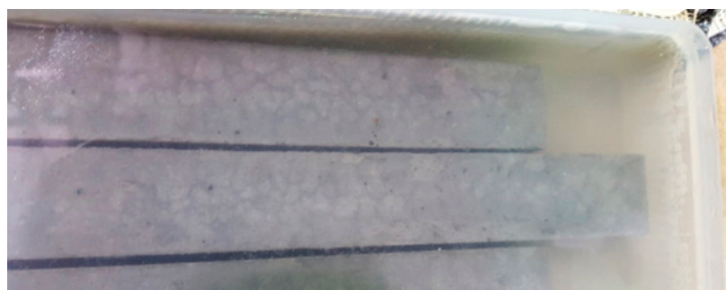
Figure 16. AAM samples for the ASR test (ASTM C1260) in a 1 N NaOH solution.
