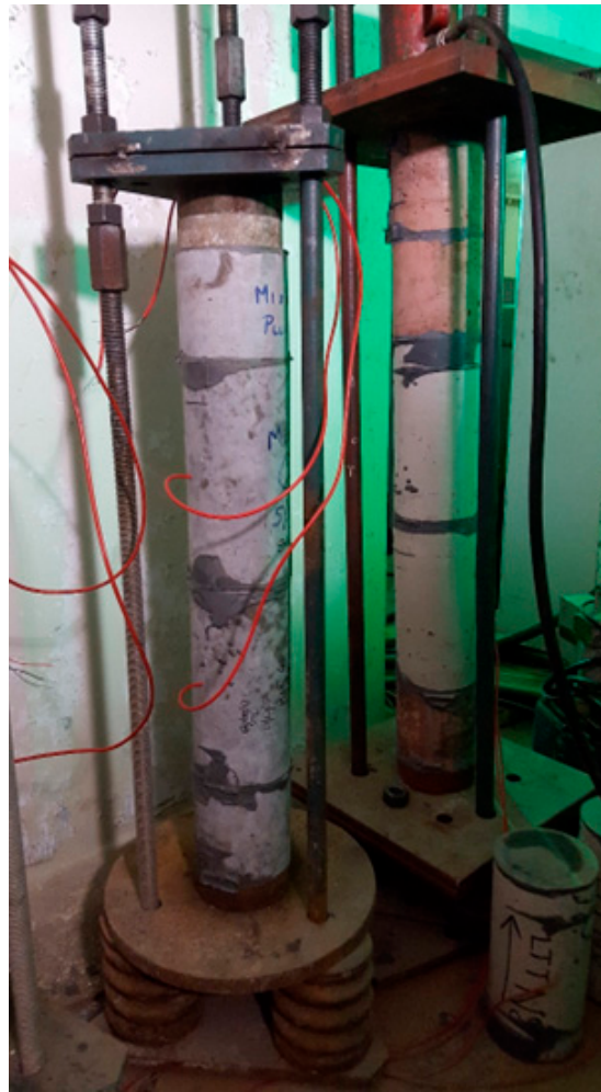
Figure 11. Creep testing setup.
