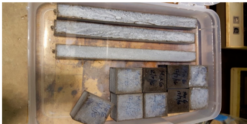
Figure 9. Test setup for sulfate-exposure testing.
