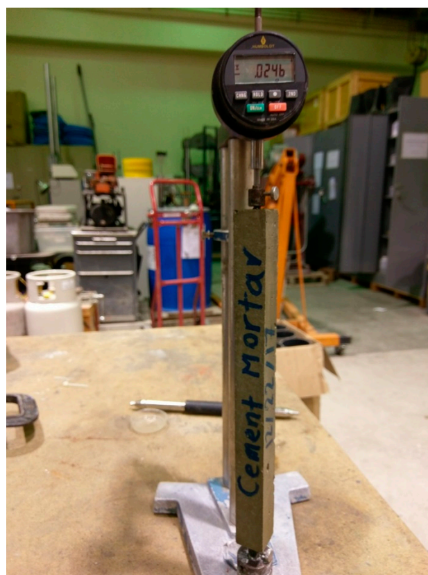
Figure 10. Test setup for potential alkali-silica reaction testing.
