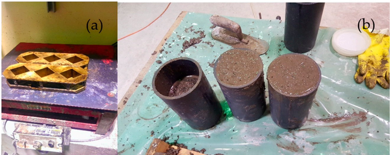
Figure 4. (a) brass mold to fabricate the mortar samples. (b) PVC mold to fabricate the concrete samples.
