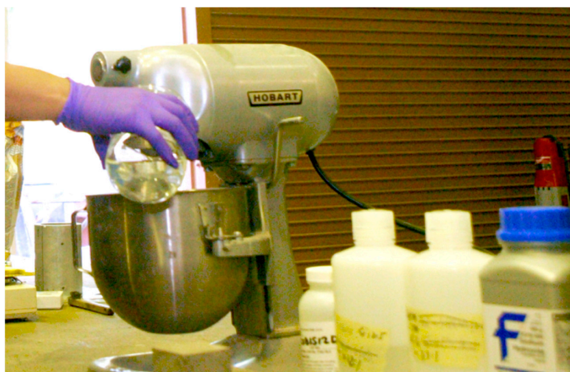
Figure 1. The mixer (Hobart N50 mixer with 50 qt capacity with three speeds) used to fabricate the mortar samples.
