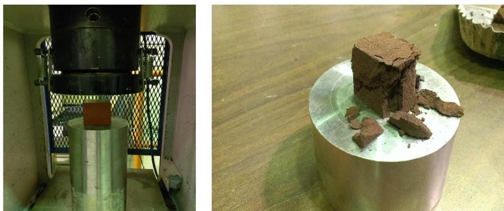
**Figure 4.** Compressive strength test of red-mud-based samples.
