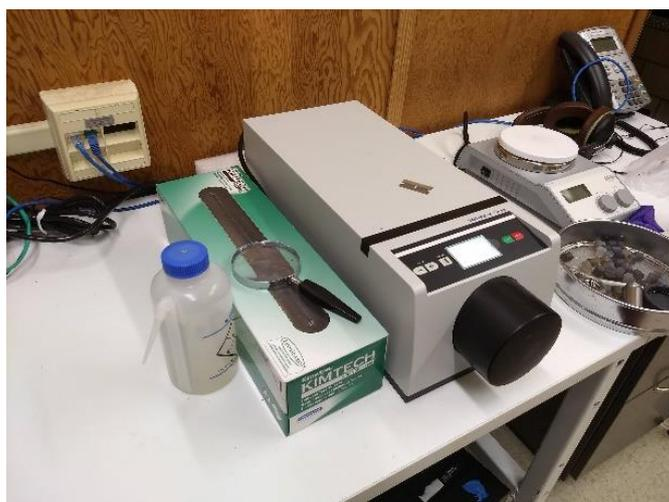
**Figure 6.** XRD sample preparation (5 µm mill).
