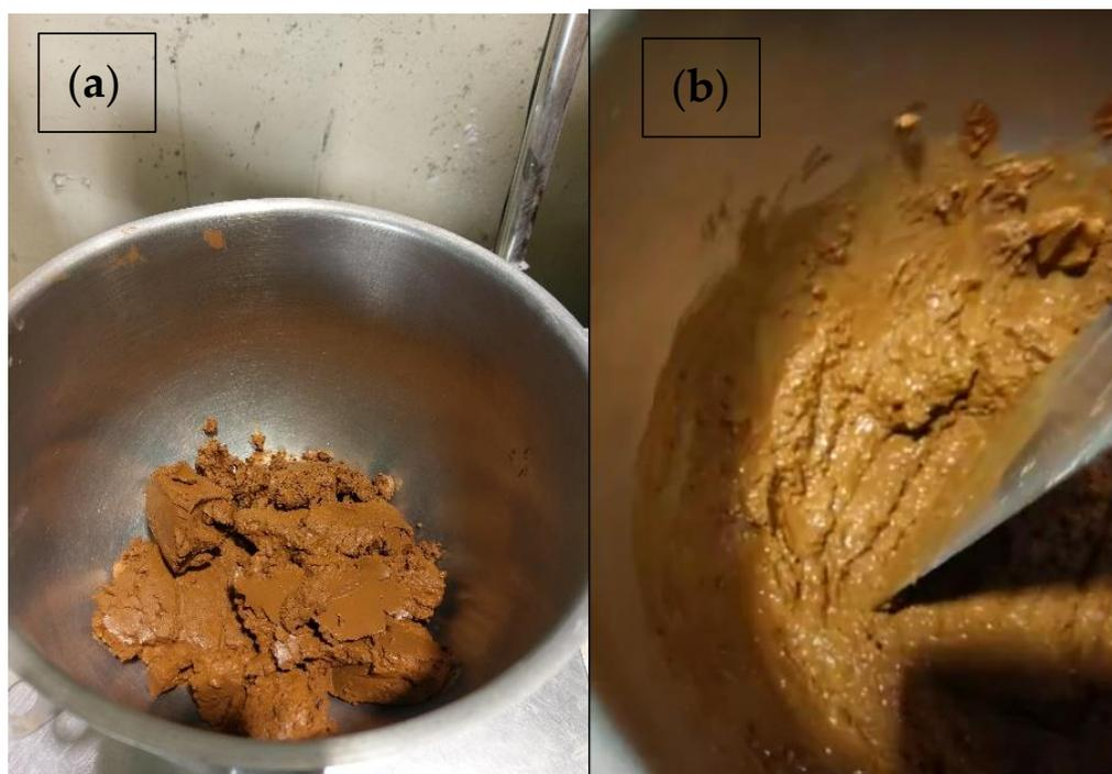
**Figure 2.** Mortar sample mixing procedure: (a) Dissolution of red mud and slag in 6 N NaOH; (b) Final red-mud-based AAM.
